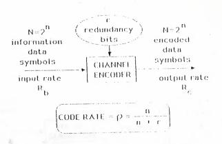
Fig: -3;10° The principle of channel encoding.
