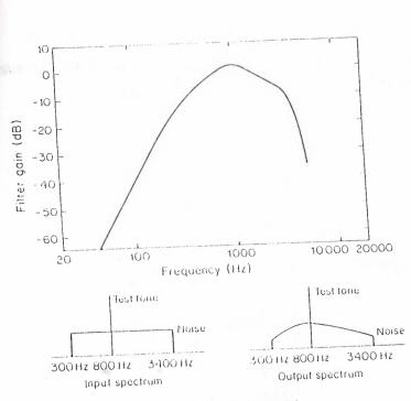
Fig **3.2**. The gain of a psophometric filter and its effect on noise.
