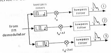
Fig. 3.6 The principle of FDM multiplexing and demultiplexing.
