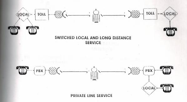
Fig. 4-5 Commercial Telephone Service Can Be Obtained Either Through Public Switching Facilities or Through Dedicated Private Lines
