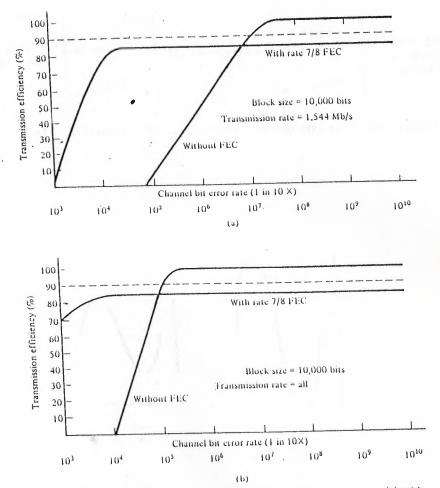
Fig . 7.13 Effect of rate 7/8 FEC code on transmission efficiency: (a) with restart-after-error detection protocol; (b) with continuous protocol with selective repeat.
