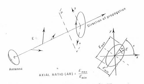
Characterisation of the polarisation of an electromagnetic wave. Fig: 2.2
