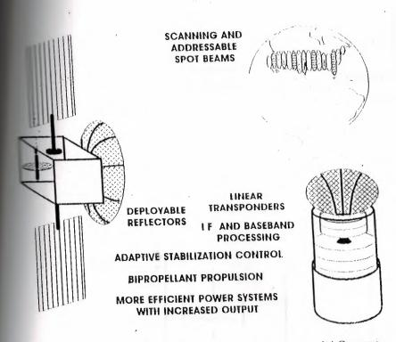
Fig. 63 Examples of Evolving Technologies for Commercial Communications Satellites with the Three-Axis (Body Stabilized) and Duat Spin Configurations
