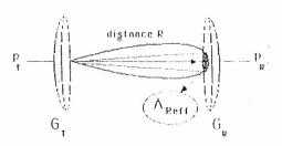
Fig 2.4. The power received by a receiving antenna
