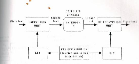
Fig. 3.9 The principle of encrypted transmission.
