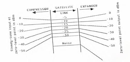
Fig: 3.5 The principle of companding.
