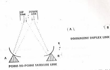
Fig. 4-1 Point-to-Point Connectivity Using a Full Duplex Satellite Link
