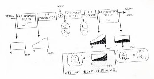
Fig: 3.4 The principle of pre- and de-emphasis.
