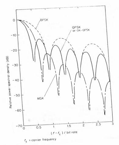
Fig. 3.14 The spectrum of digital carriers.
