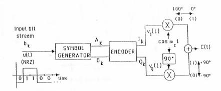
Fig: 3.13 Four-state phase modulator (QPSK).
