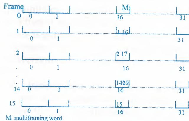
**Figure(28).** Structure of the channel associated signaling scheme for the 30-channel PCM system
