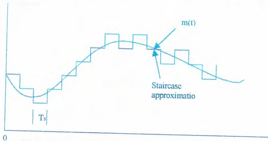
Figure(19). Illustration of delta modulation
