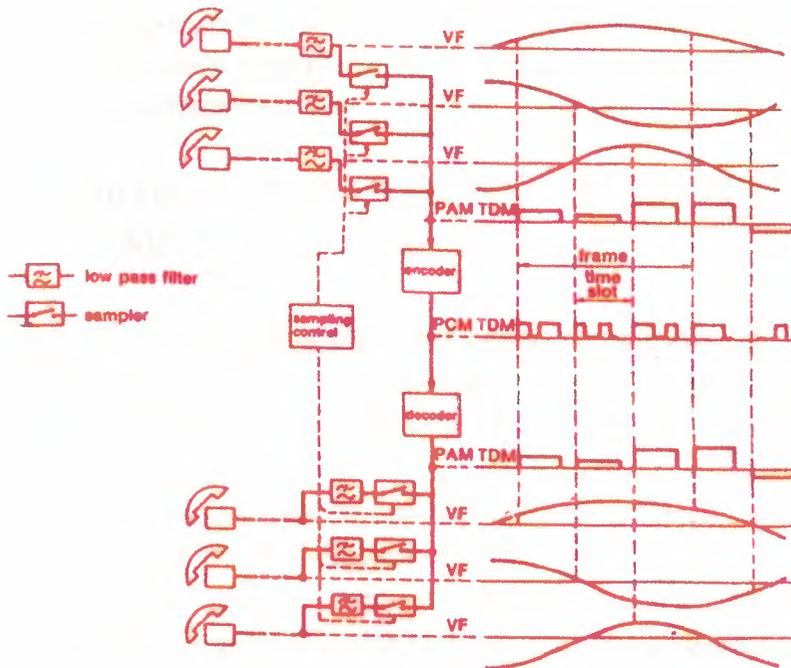
Figure(24) A PAM transmission system using time division multiplex (TDM)
