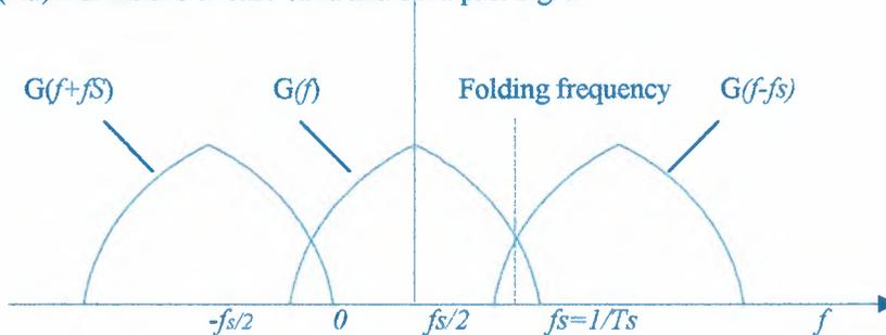
Figure (7.b) spectrum of under sampled information signal showing interference between spectral replicas and the folding frequency
