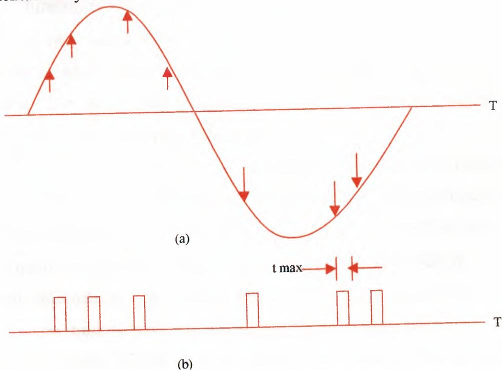
Figure(22.a.b) pulse frequency modulation PFM(a) modulating signal.(b)modulated pulse train
