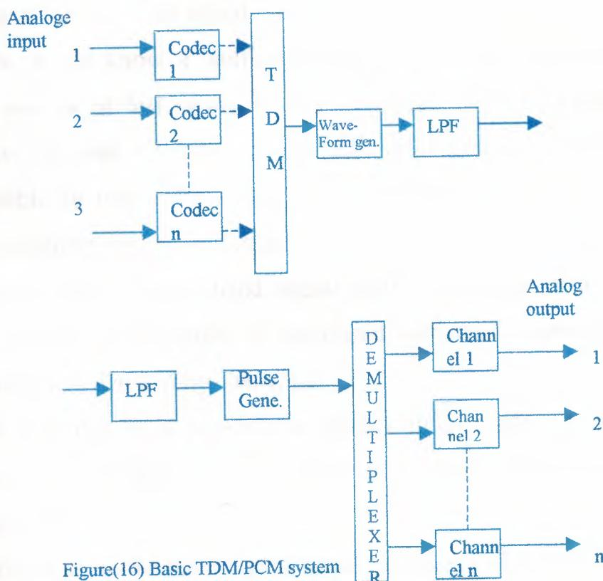
Figure(16) Basic TDM/PCM system
