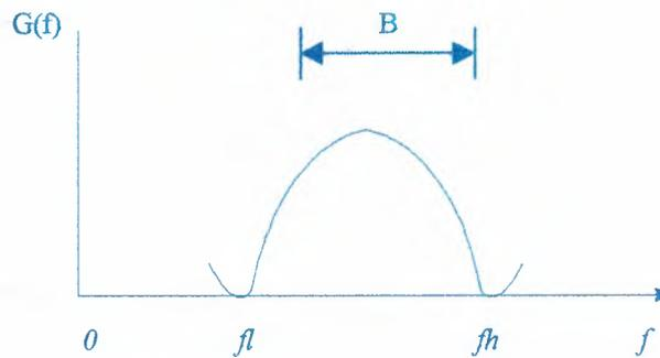
Figure (7.a) Definitions of base band and band pass signal
