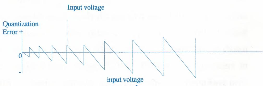
Figure(14.a.b) Nonlinear quantization
