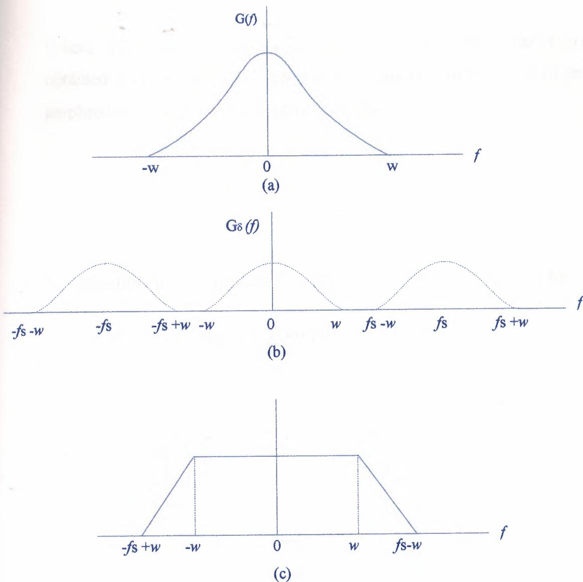
**Figure 1.** (a) Pre-alias filtered spectrum of an information-bearing signal. (b) Spectrum of instantaneously samples version of the signal, assuming the use of a sampling greater than the Nyquist rate. (c) Amplitude response of reconstruction filter.
