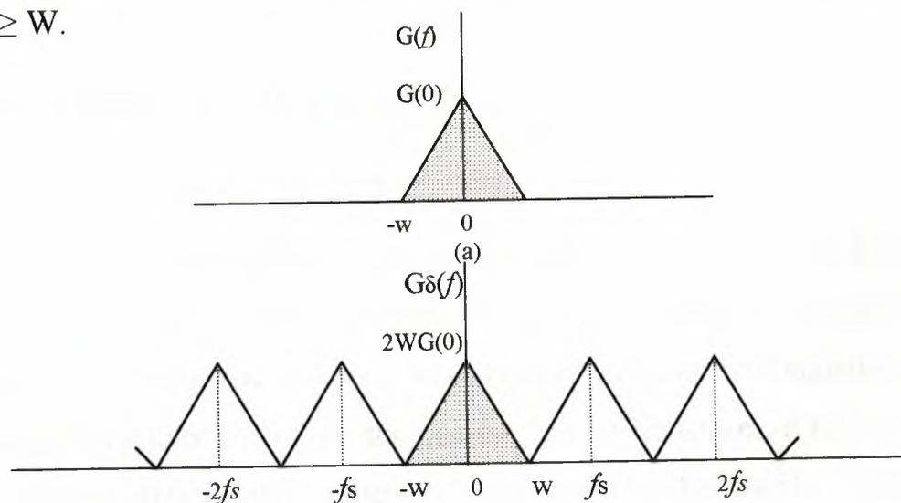
**Figure (5).** (a) Spectrum of a strictly band limited signal  $g(t)$ . (b) spectrum of sample version of  $g(t)$  for a sampling period  $T_s=1/2w$ .
