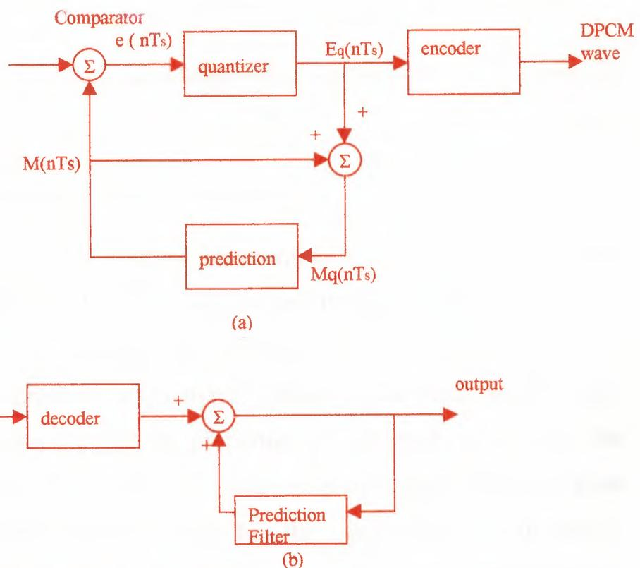
Figure (17) DPCM system. (a)transmitter. (b)receiver.
