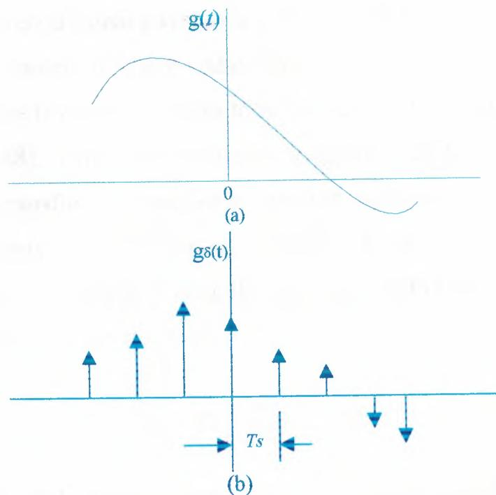
**Figure (4).** The sampling Process (a) analog signal. (b) instantaneously sampled version of the signal.
