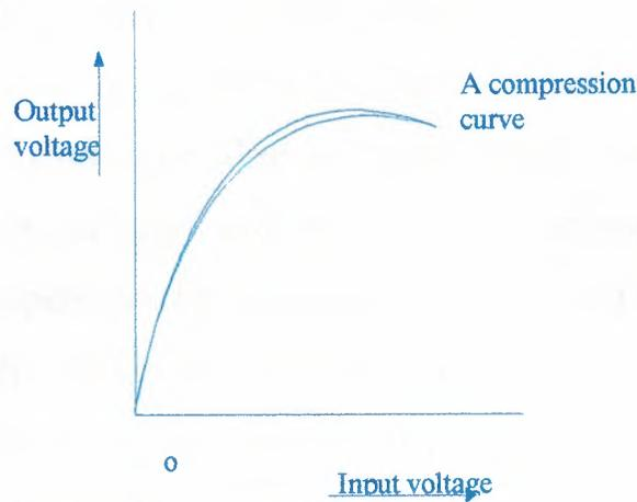
Figure(13) chorded approximation to a compression curve
