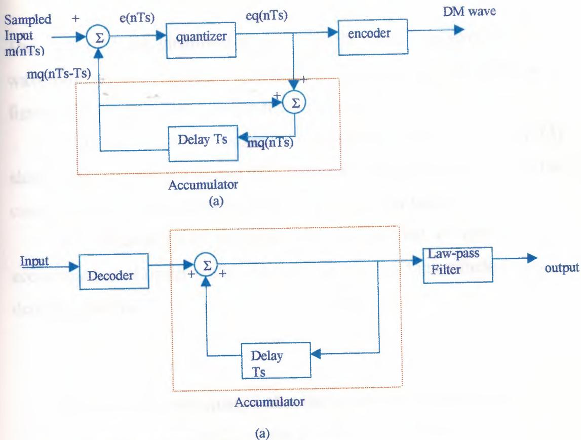
Figure(20). DM system. (a)Transmitter(b) Receiver
