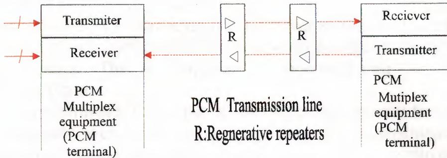
Figure(26) Two multiplex equipment units
