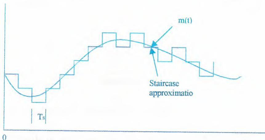
Figure(19). Illustration of delta modulation
