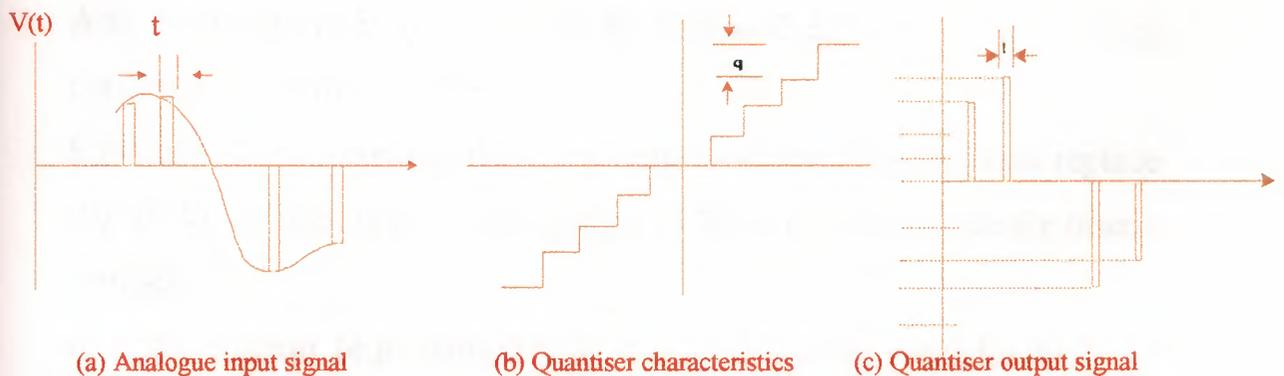
Figure(9) Quantisation of a PAM signal.
