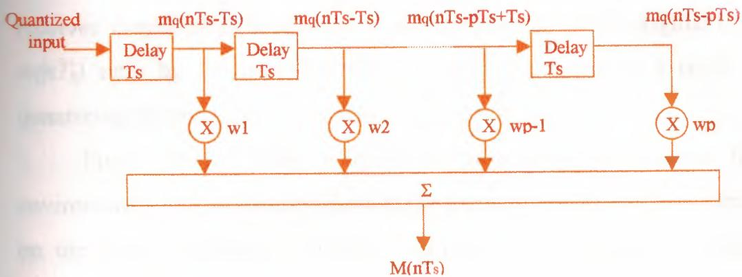
**Figure(18).** Tapped-delay-line filter used as a prediction filter
