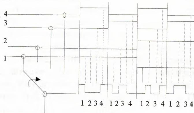
Figure(30). Bit interleaving
