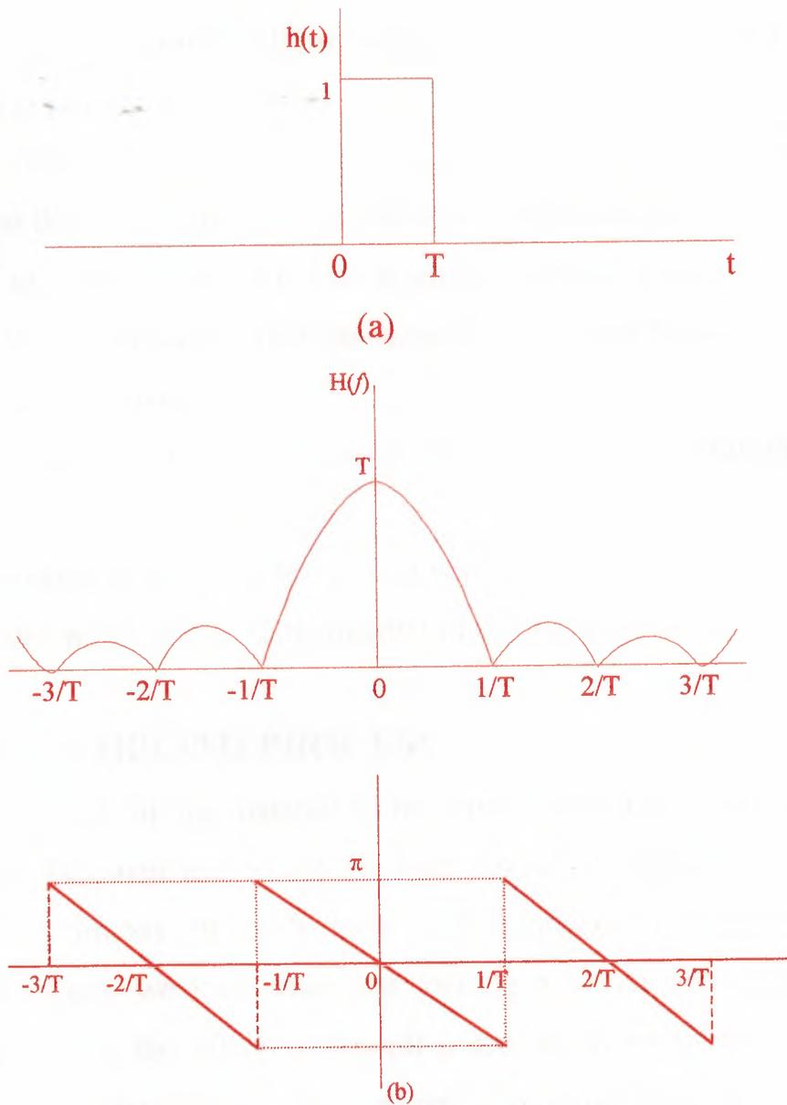
**Figure 3.** (a) rectangular pulse  $h(t)$ , (b) spectrum  $H(f)$
