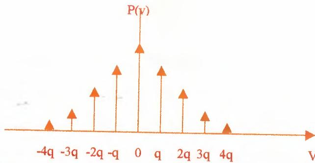
Figure (10) Discrete pdf of quantised PAM signal
