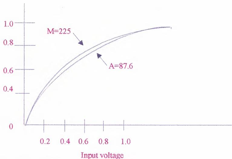
Figure(12) compressor characteristics for  $\mu=255$  and  $A=87.6$
