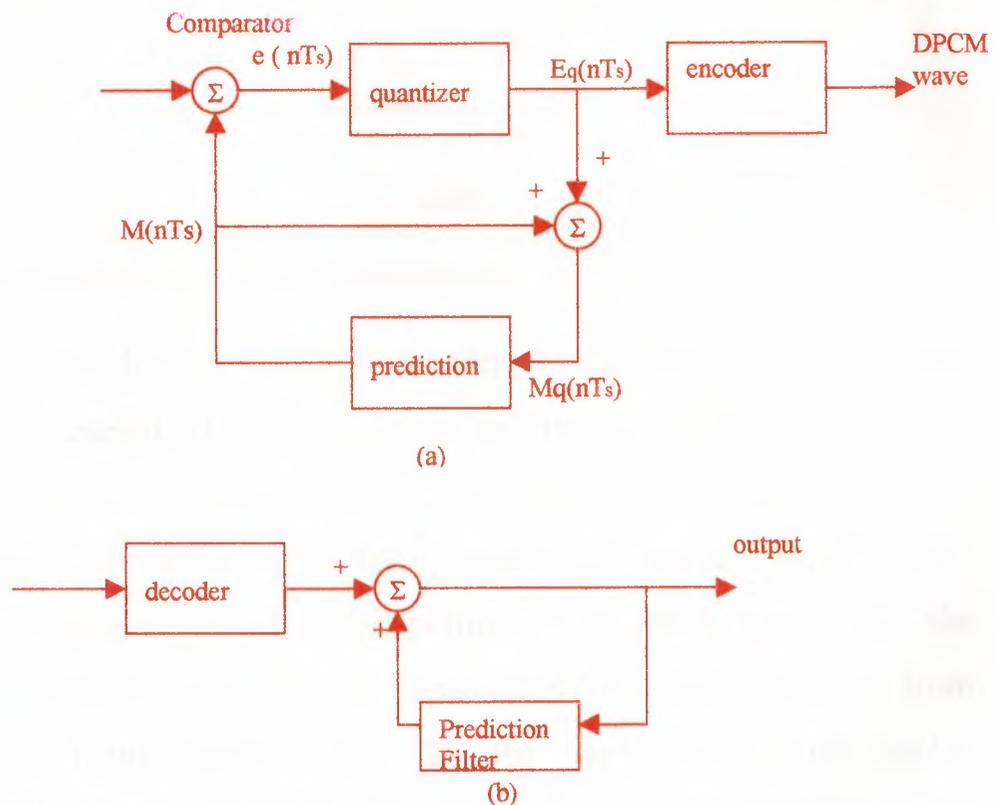
Figure (17) DPCM system. (a)transmitter. (b)receiver.
