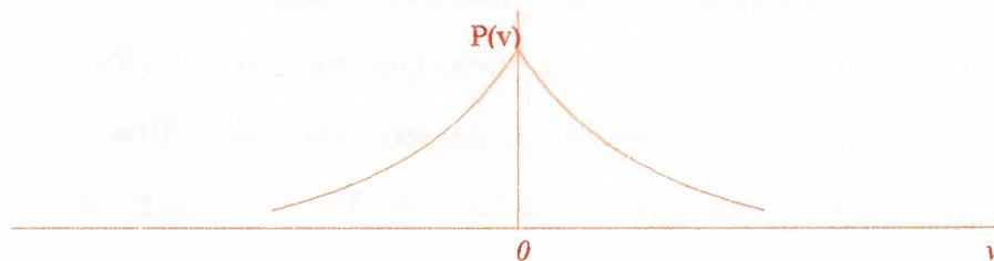
Figure(8) Continuous pdf of typical analogue PAM signal
