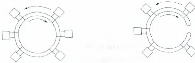
Fig. 5.4. (a) FDDI consists of two counter rotating rings, (b) In the event of failure of both rings at one point, the two rings can be joined together to form a single long ring.
