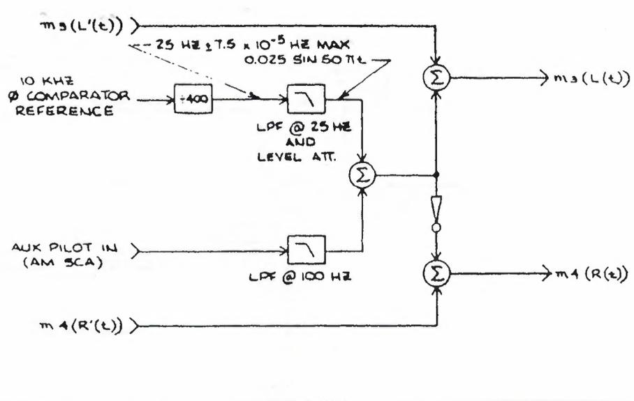
FIGURE 1.4. PILOT TONE AND AM SCA INSERTION CIRCUITRY
