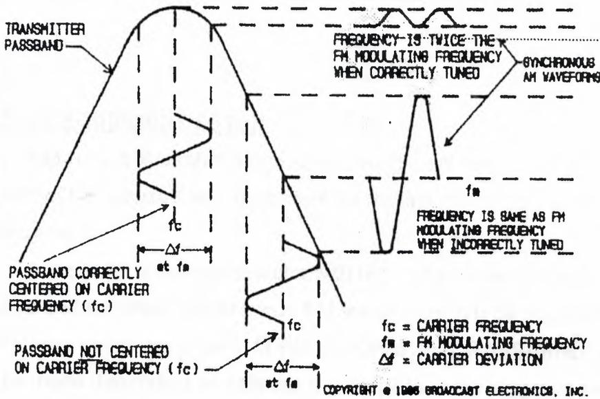
Figure 6.1 SYNCHRONOUS AM WAVEFORMS AND CALCULATIONS
