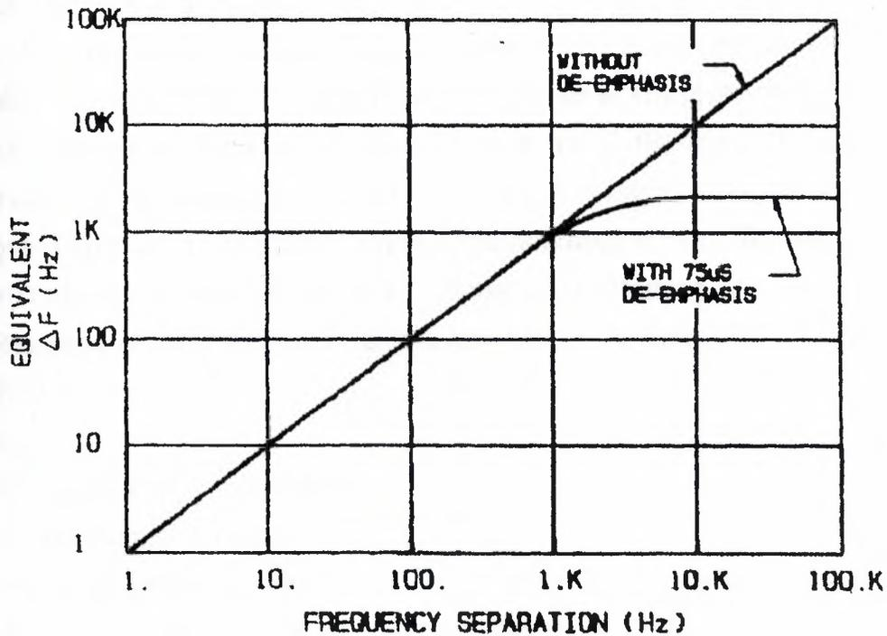
Fig.7 RELATIONSHIP OF CARRIER FREQUENCY SEPERATION TO EQUIVALENT CARRIER FREQUENCY DEVIATION ( $\epsilon=1$ )
