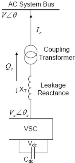
**Figure 4.1** Basic model of a StatCom
