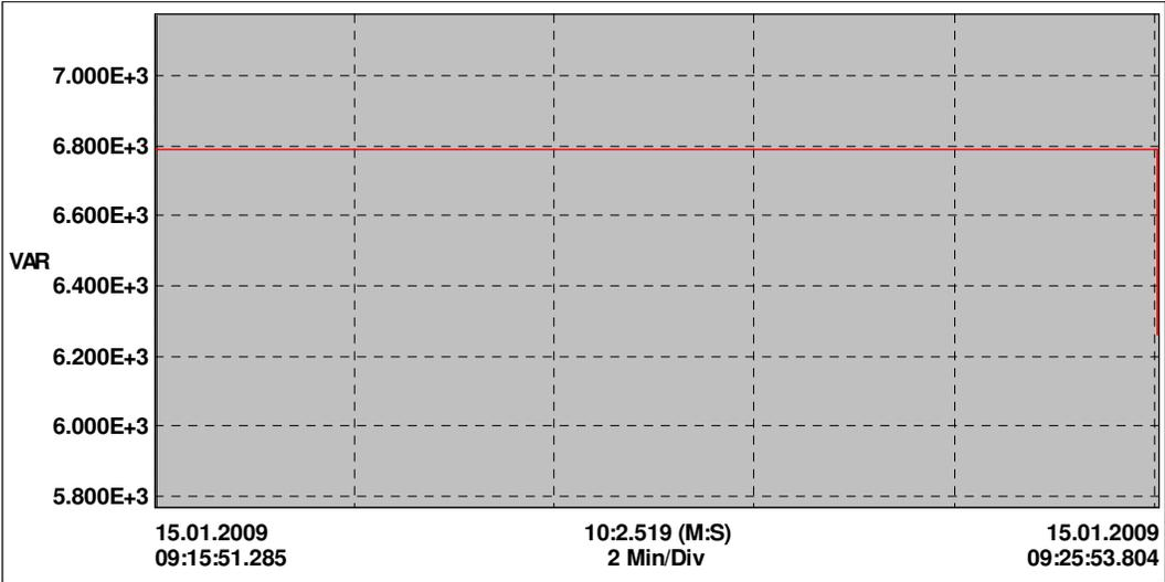
**Figure 3.60** Reactive power of line1 during compensation
