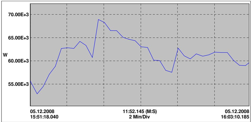
**Figure 3.25** Active power of line3 before compensation
