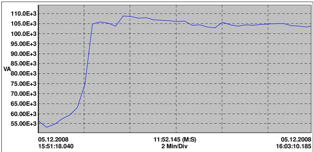
**Figure 3.29** Apparent Power of line3 before compensation
