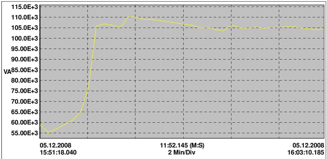
**Figure 3.28** Apparent Power of line2 before compensation
