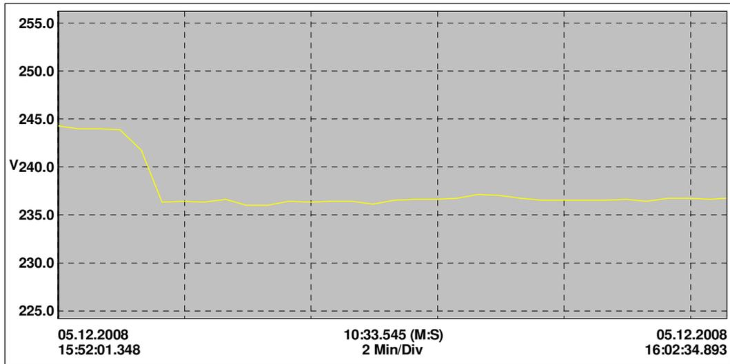
**Figure 3.10**  $V_{rms}$  of line 2 before compensation
