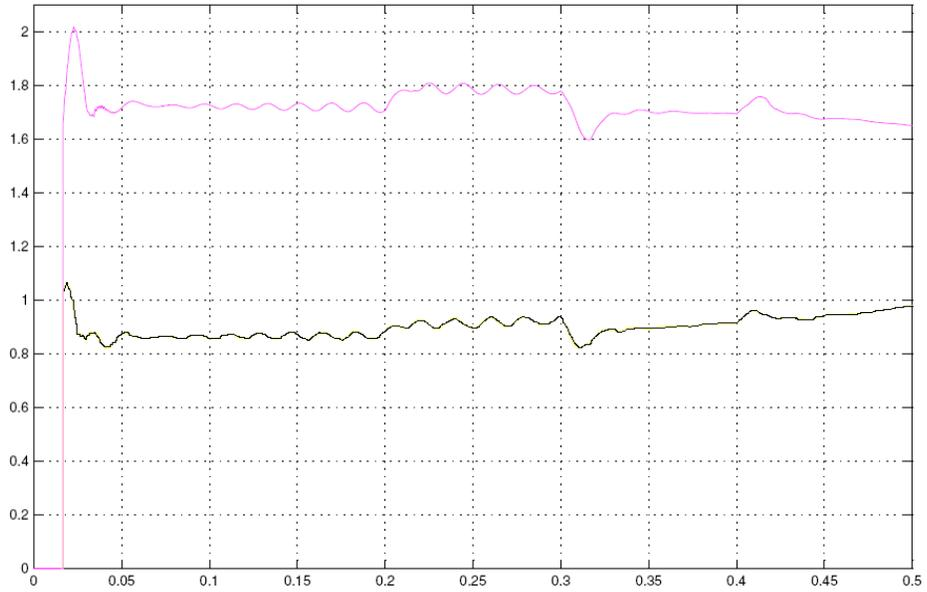
**Figure 4.4** Reactive and active powers without StatCom
