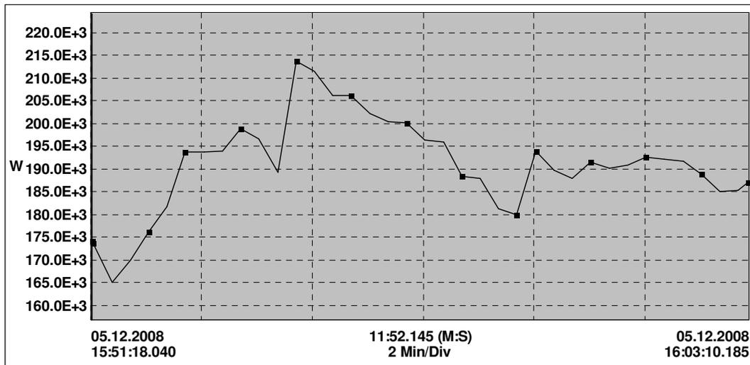
**Figure 3.26** Total active power of phases before compensation
