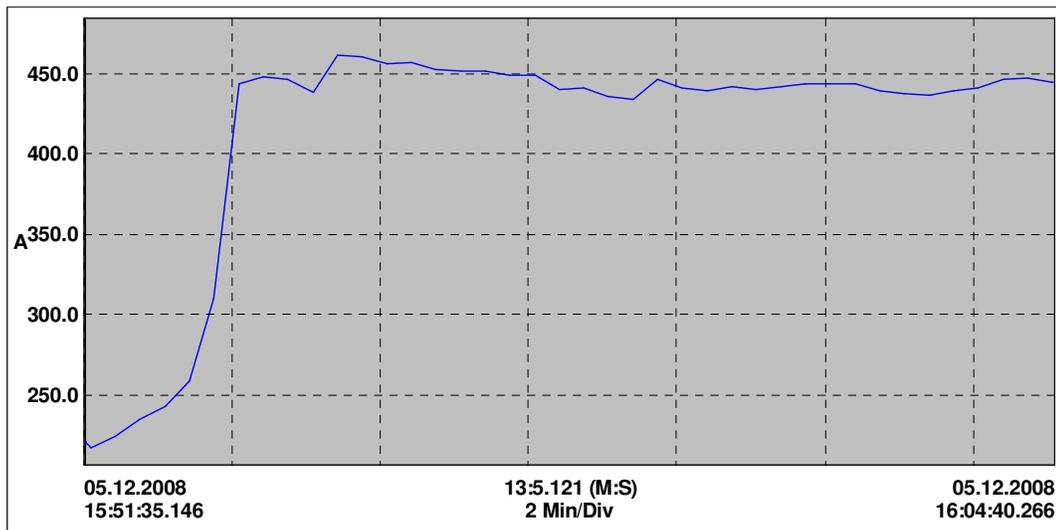
**Figure 3.14** Motor starting before compensation and results current in line 2
