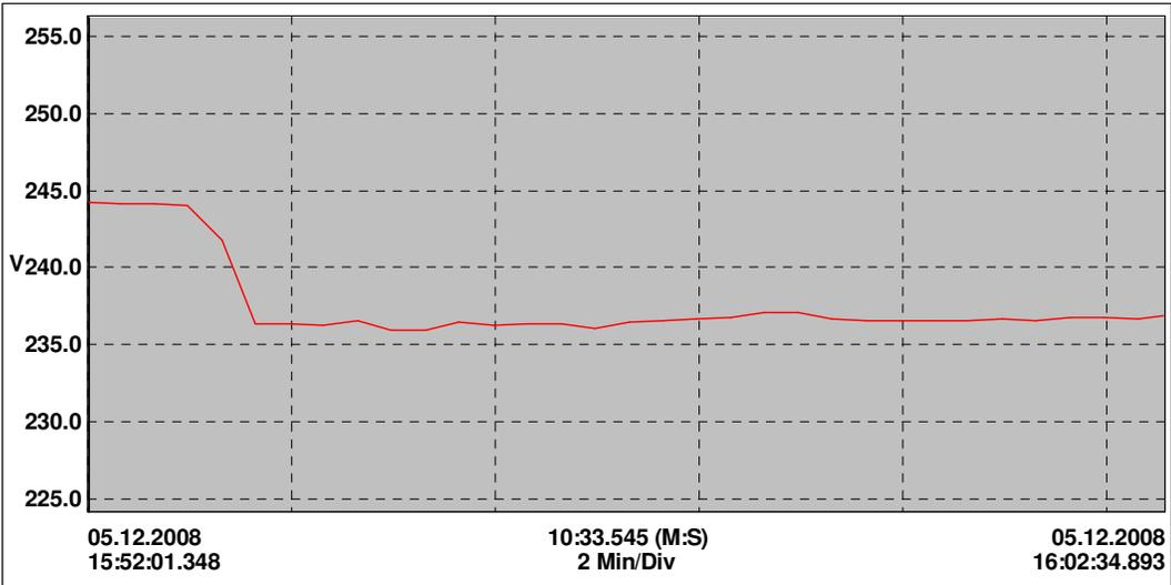
**Figure 3.9** V<sub>rms</sub> of line 1 before compensation
