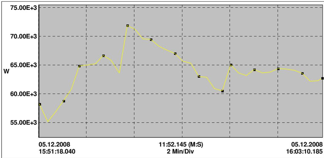
**Figure 3.24** Active power of line2 before compensation
