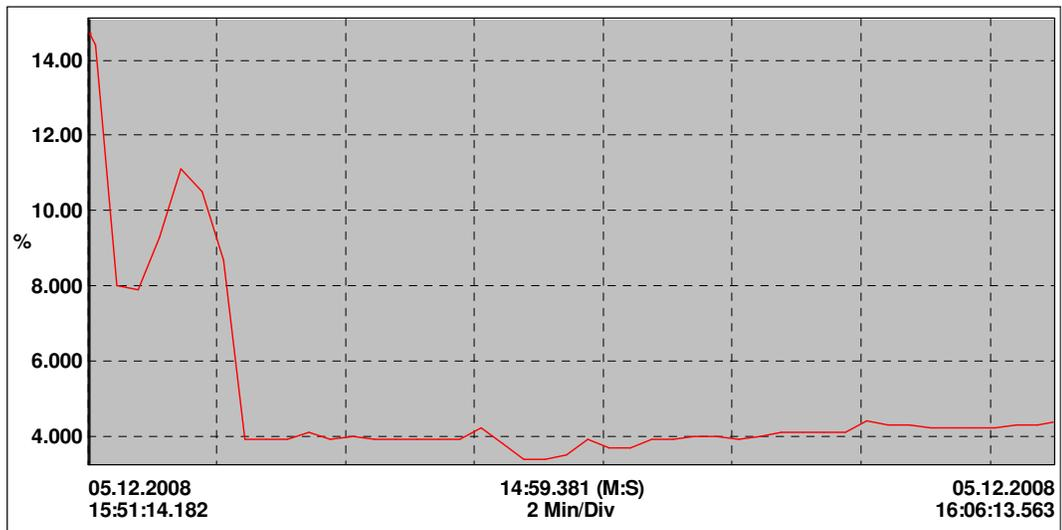
**Figure 3.19** Current THD of line1 before compensation
