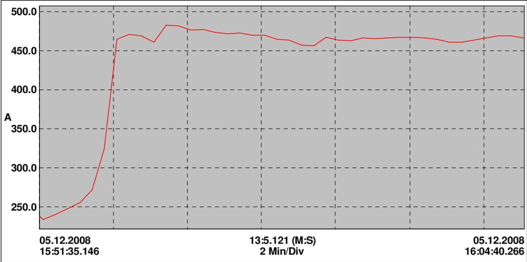
Figure 3.12 Motor starting before compensation and results current in line 1
