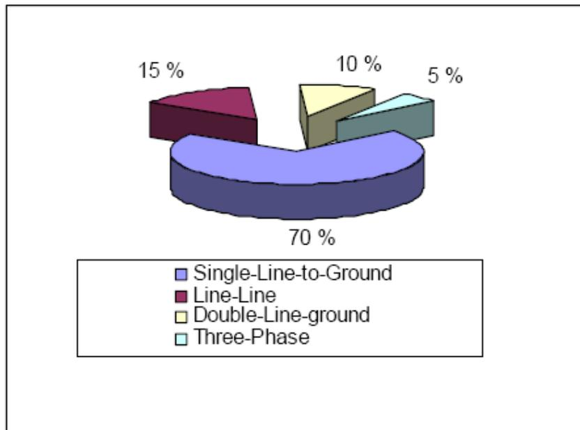
**Figure 2.6** Probabilities of voltage sag due to system faults
