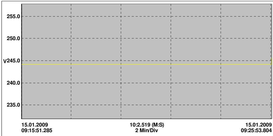
**Figure 3.40**  $V_{rms}$  of line2 during Compensation
