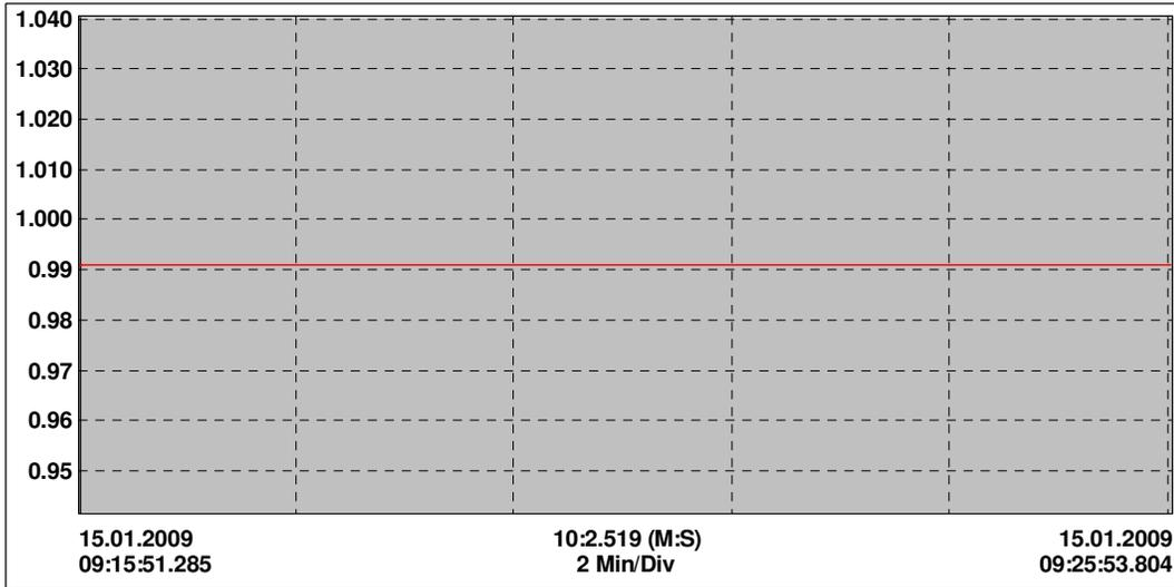
**Figure 3.65** Power factor of line 1 during compensation
