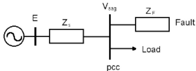
**Figure 2.5** Voltage divider model for voltage sag caused by a system fault
