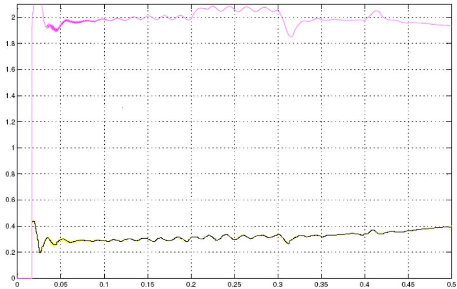
**Figure 4.5** Reactive and active powers with StatCom
