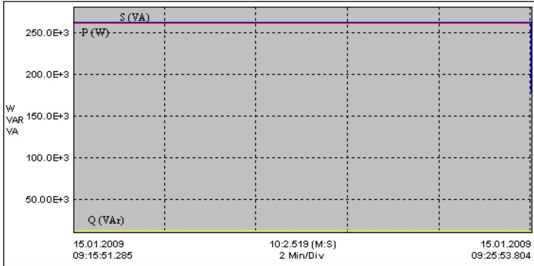
**Figure 3.64** Active, Apparent and Reactive power at the system terminal with compensation  $\cos\phi = 0$ .
