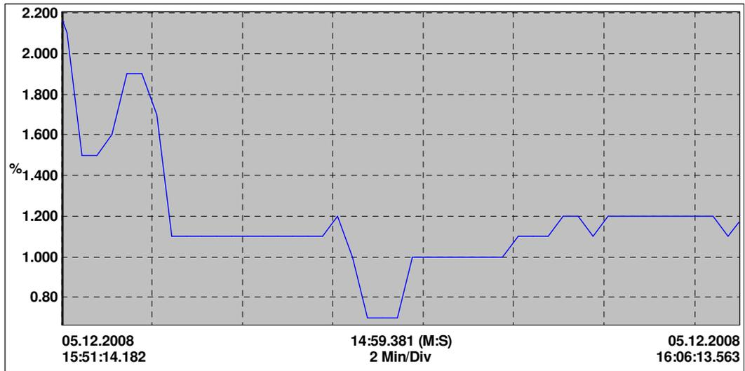
**Figure 3.18** Voltage THD of line3 before compensation
