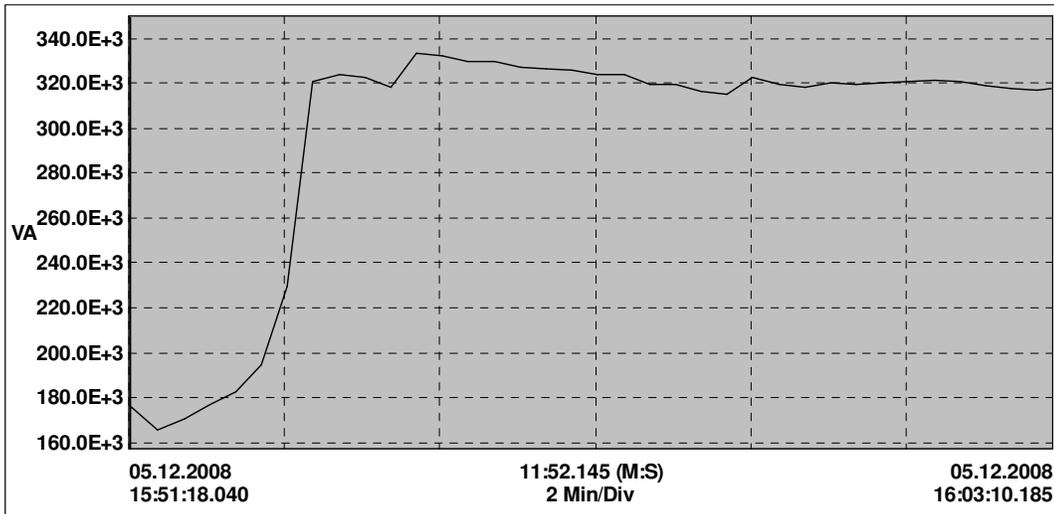
**Figure 3.30** Total apparent Power of phases before compensation
