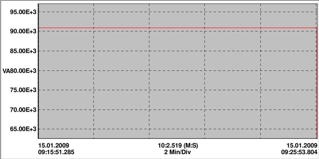
Figure 3.56 Apparent power of line1 during compensation
