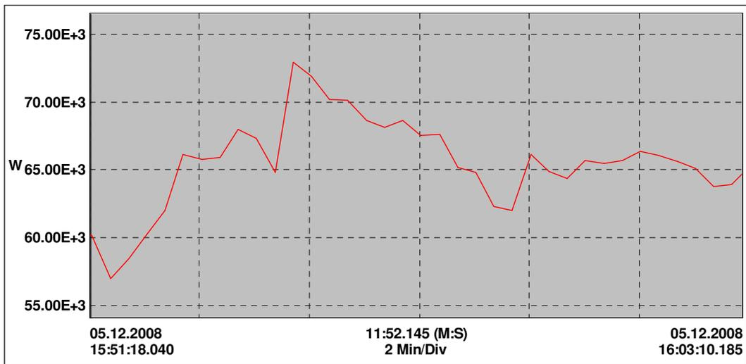
**Figure 3.23** Active power of line1 before compensation
