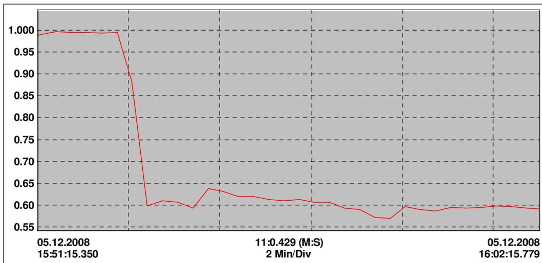
**Figure 3.35** Power factor of line 1 before compensation
