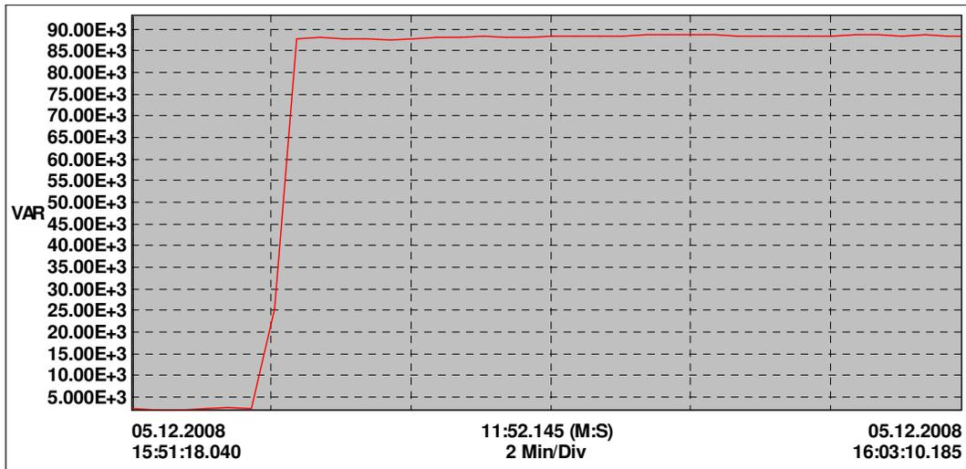
**Figure 3.31** Reactive power of line 1 before compensation
