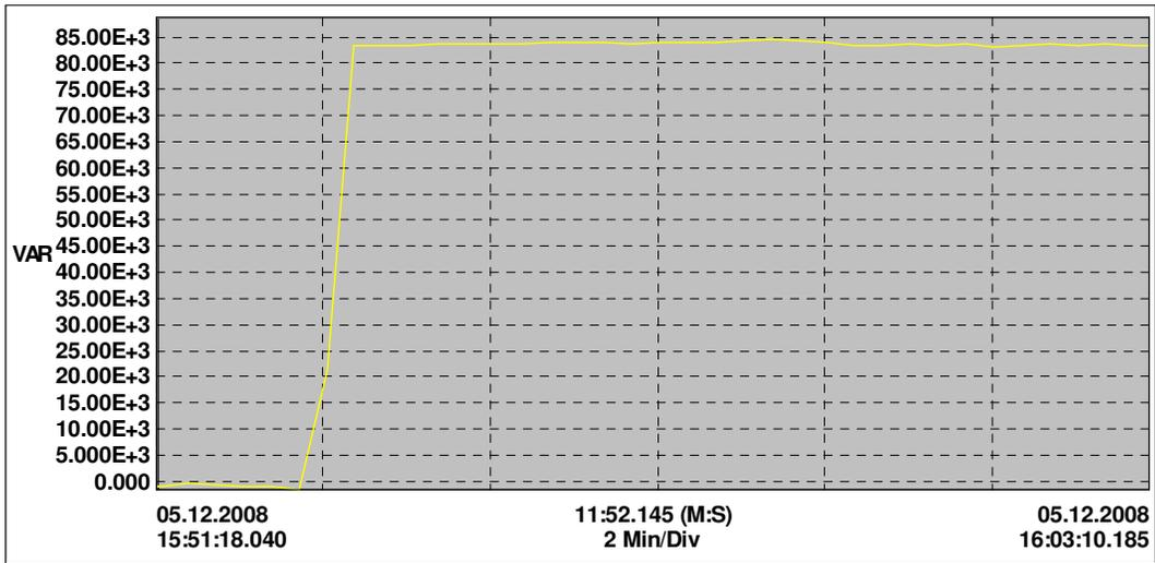
**Figure 3.32** Reactive power of line 2 before compensation
