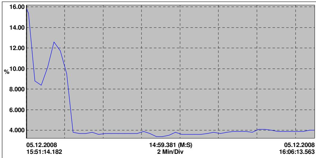
**Figure 3.21** Current THD of line3 before compensation
