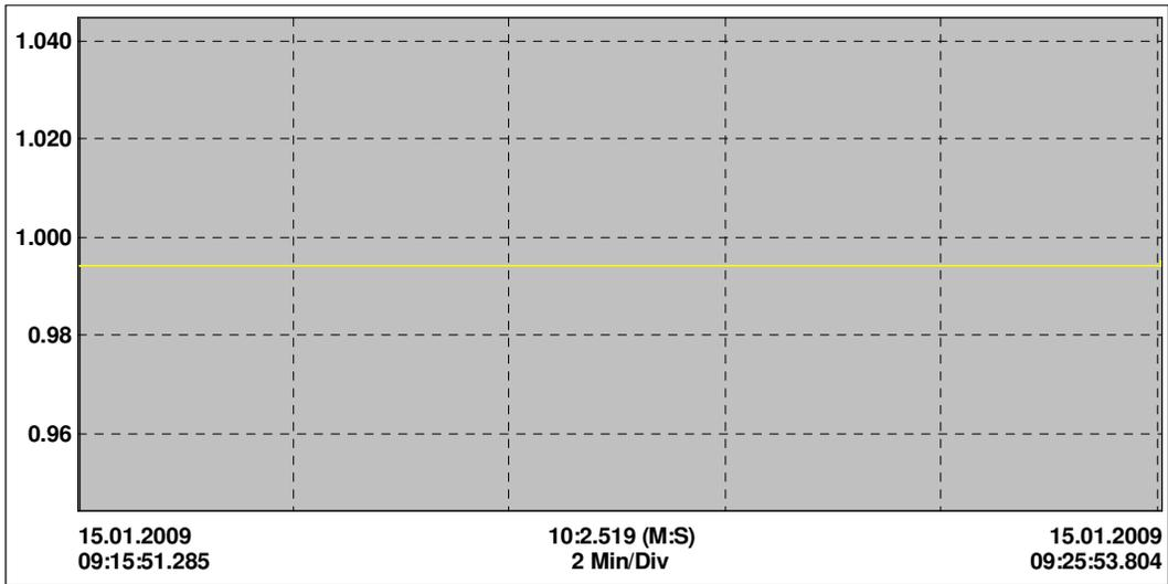
**Figure 3.66** Power factor of line 2 during compensation
