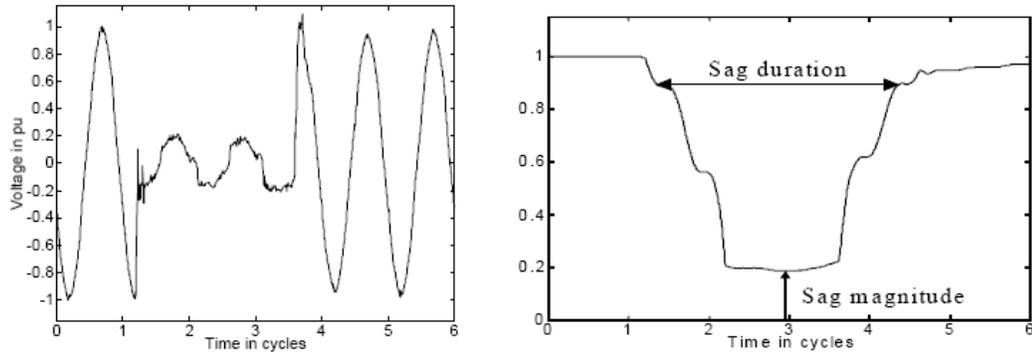
**Figure 2.2** The voltage sag phenomena in one phase
