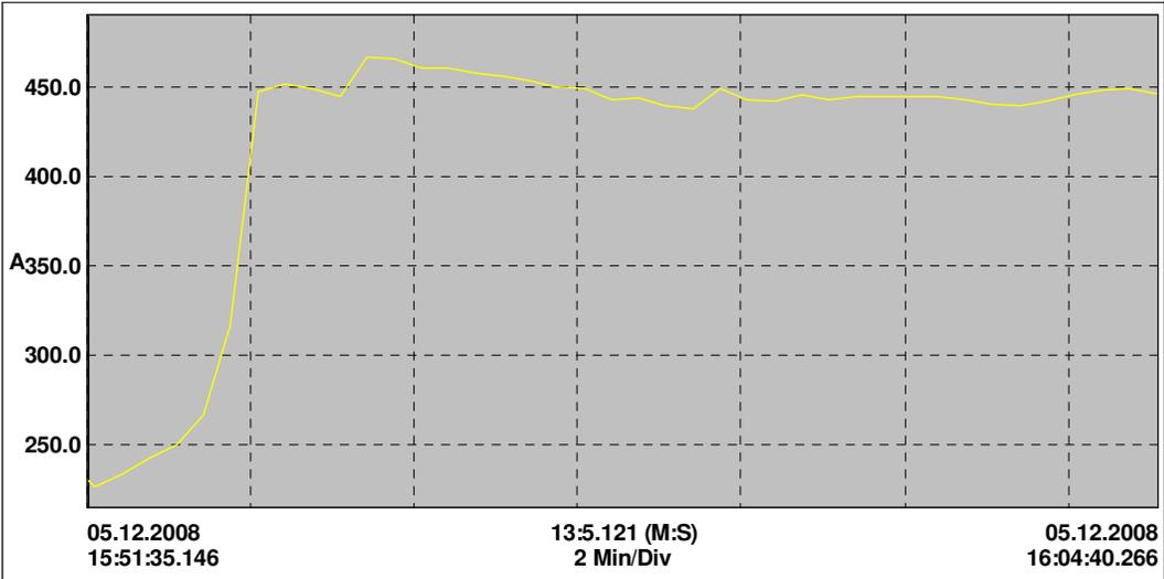
Figure 3.13 Motor starting before compensation and results current in line 2
