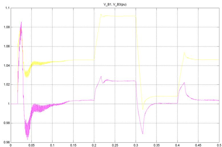
**Figure 4.7** Load bus voltage with StatCom
