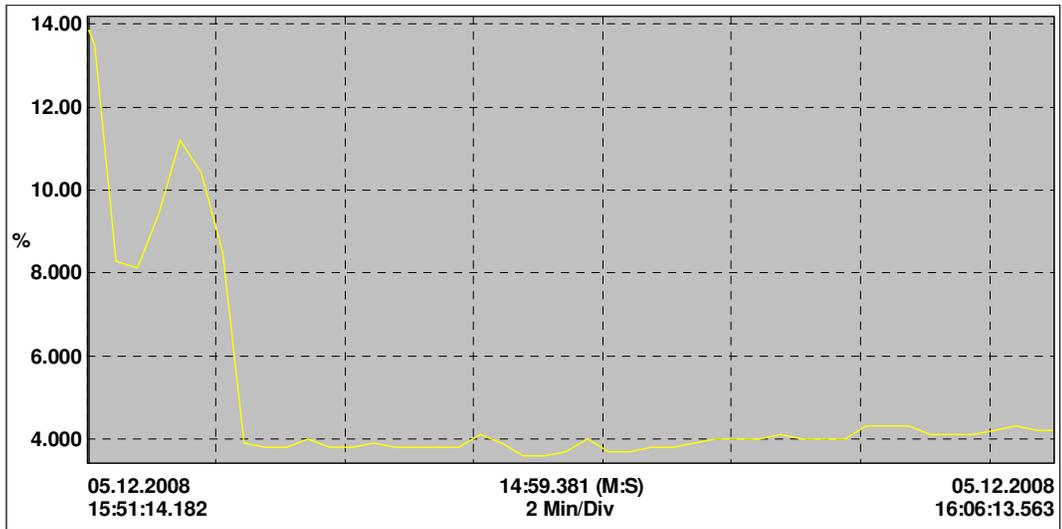
**Figure 3.20** Current THD of line2 before compensation
