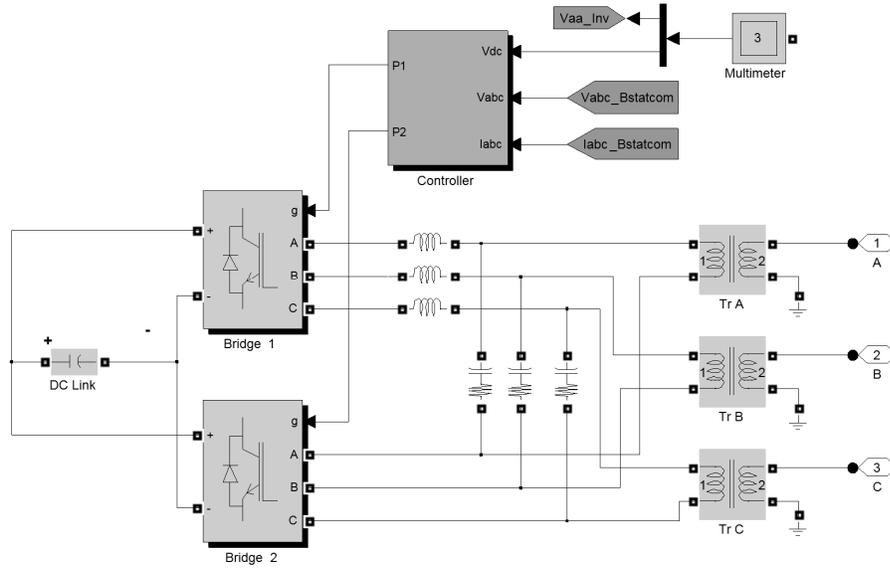
**Figure 4.2** Control scheme of the StatCom
