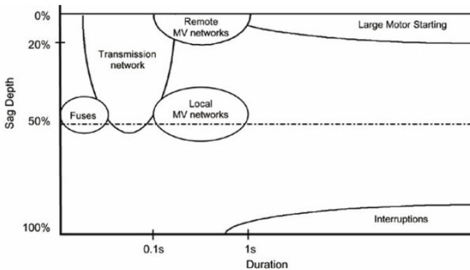
**Figure 2.4** Sag depth Vs duration plot
