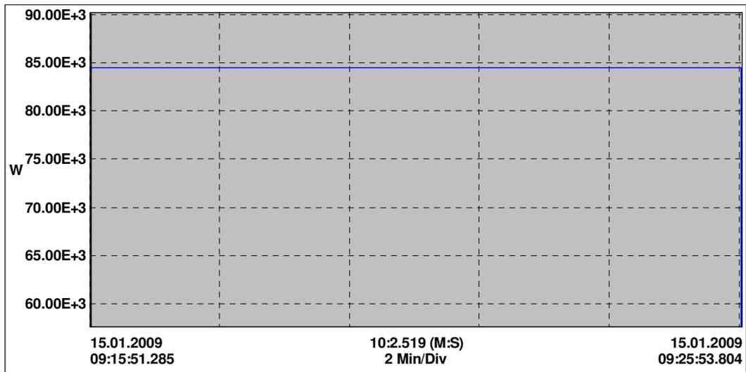
**Figure 3.54** Active power of line3 during compensation
