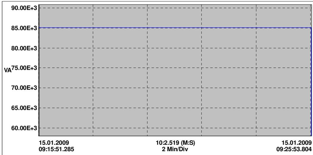
**Figure 3.58** Apparent power of line3 during compensation
