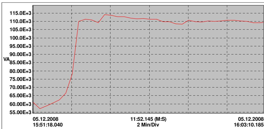
**Figure 3.27** Apparent Power of line1 before compensation
