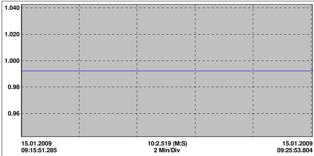
**Figure 3.67** Power factor of line 3 during compensation
