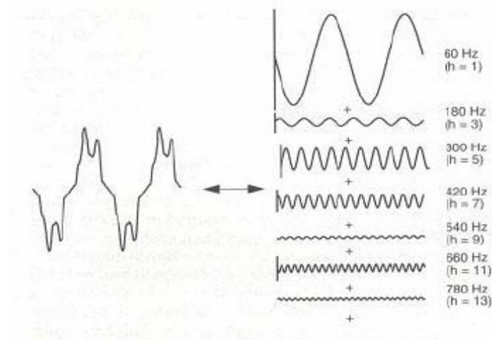
**Figure 2.8** Fourier series representation of a distorted waveform
