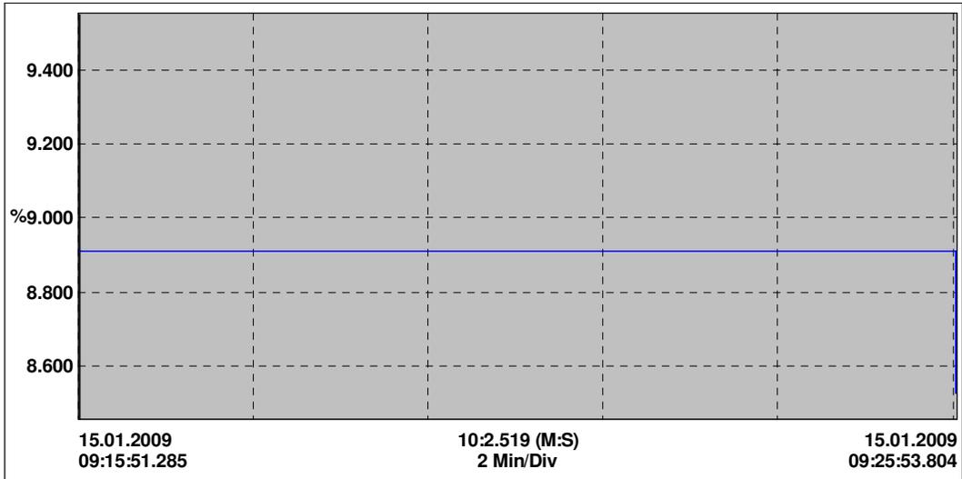
Figure 3.51  $I_{thd}$  of line3 during compensation
