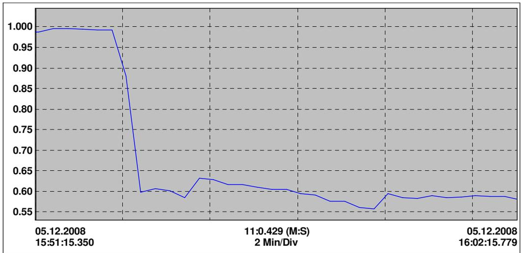
**Figure 3.37** Power factor of line 3 before compensation
