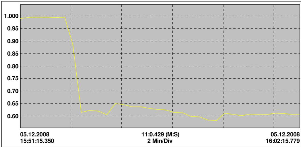
**Figure 3.36** Power factor of line 2 before compensation
