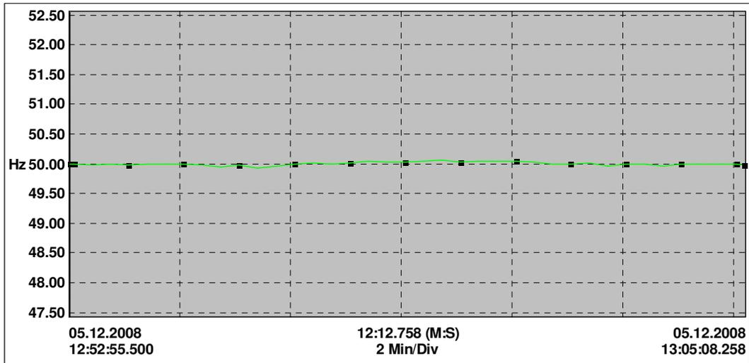
**Figure 3.22** Bus frequency before compensation
