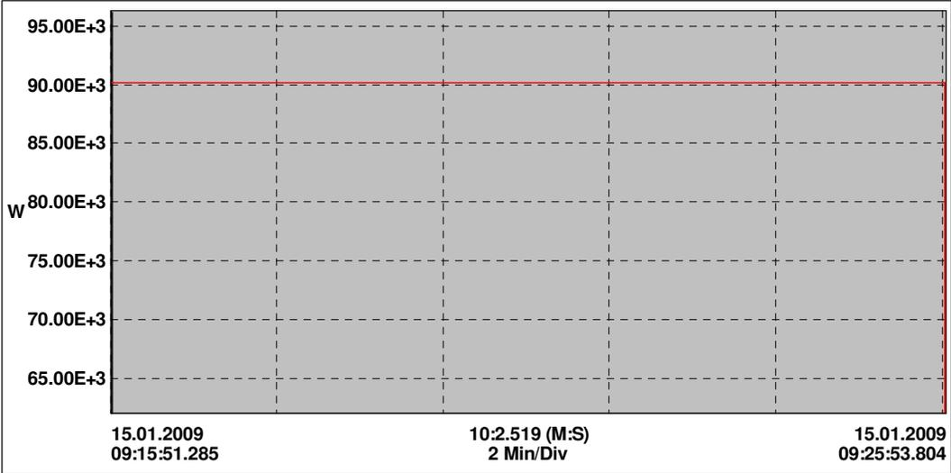
Figure 3.52 Active power of line1 during compensation
