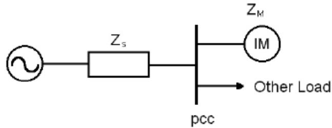
**Figure 2.7** Equivalent circuit for induction motor starting
