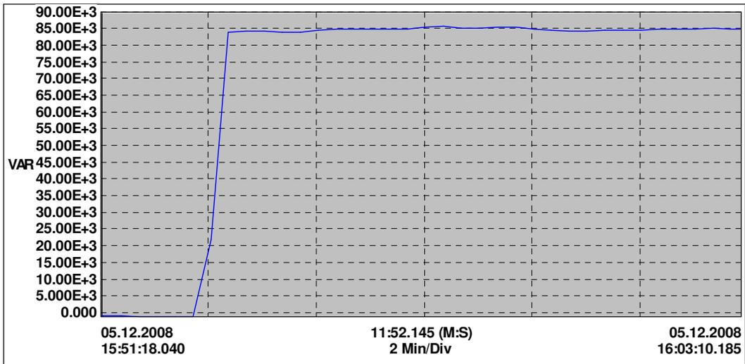
**Figure 3.33** Reactive power of line 3 before compensation
