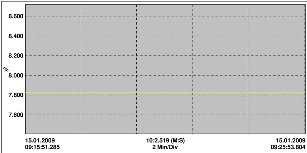
Figure 3.50  $I_{thd}$  of line2 during compensation
