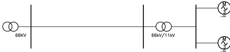
**Figure 3.1** Bozkaya single line diagram
