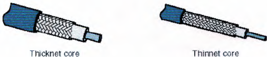
Figure 2.5 Thicknet cable has a thicker core than thinnet cable
