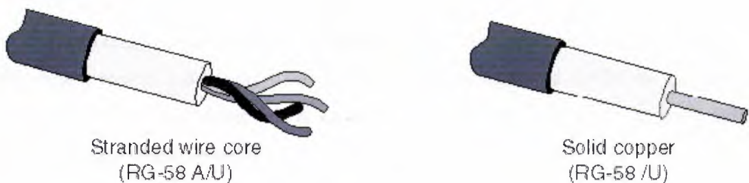
Figure 2.4 RG-58 coaxial cable showing stranded wire and solid copper cores
