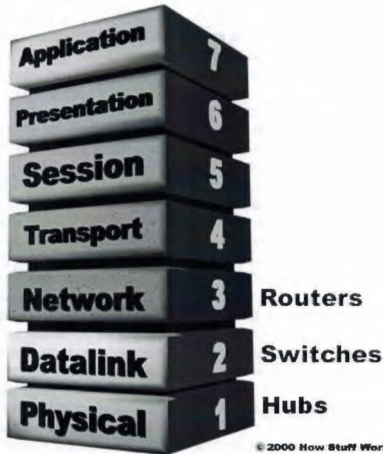
figure : The OSI Reference Model consists of seven layers that build from the wire (Physical) to the software (Application).
