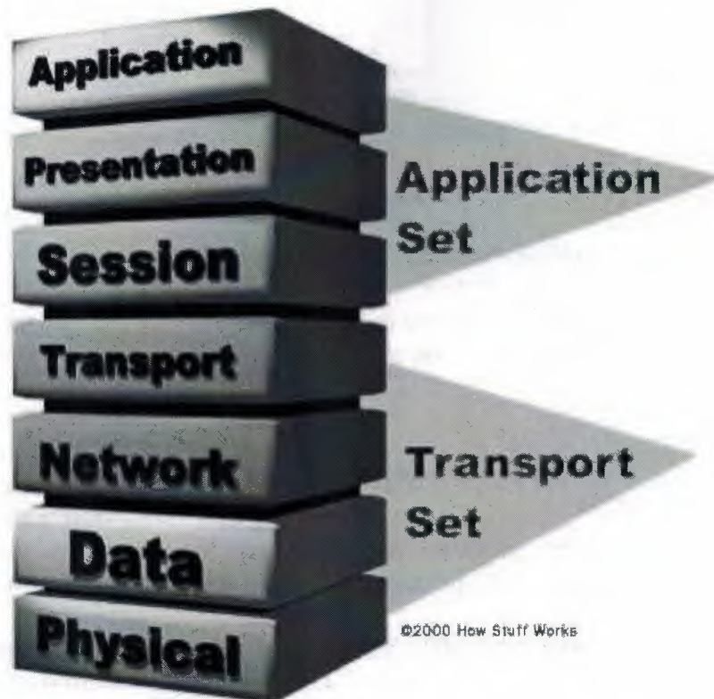
figure :The seven layers of the OSI Reference Model
