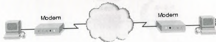
Figure 1.9 Shows a Simple modem-to-modem connection
