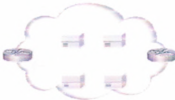
Figure 1.5: Shows Two Routers of a WAN Connected by Switches
