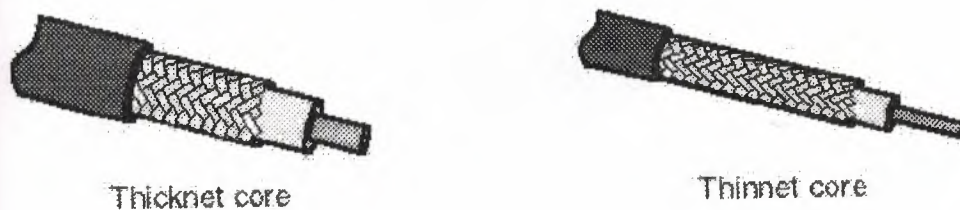
Figure 2.5 Thicknet cable has a thicker core than thinnet cable
