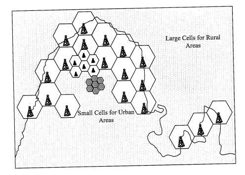
Figure 2.6. Cell Splitting
