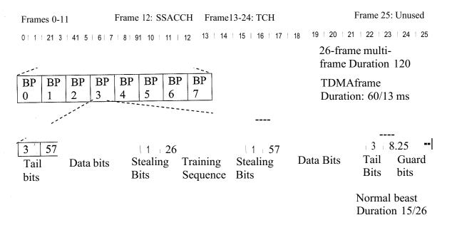
Figure 3.2.0rganization ofbursts, TDMA frames, and multi-frames far speech and data
