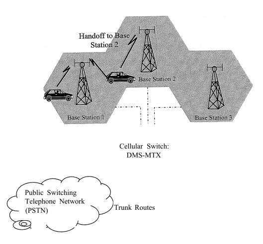
Figure 2.7. Handoffbetween Adjacent Cells
