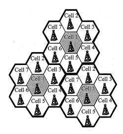
Figure 2.6. Frequency Reuse
