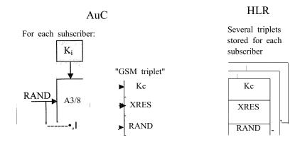
Figure 4.2 Diagram of Triplet Generation
