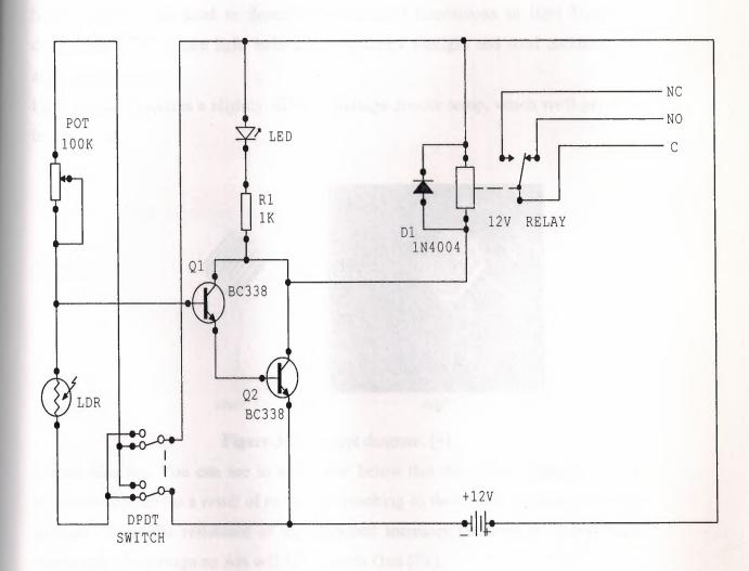
Figure 3.1 Circuit of light/Dark activated Alarm. [8]
