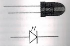
Figure 3.5 A circuit symbol of a light emitting code and
