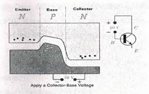
Figure 1.14: The applying collector-base voltage. [6]
