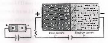
Figure 1.9: Forward Biased P-N Junction. [5]
