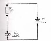
Figure 3.5 A LED connections diagram.
