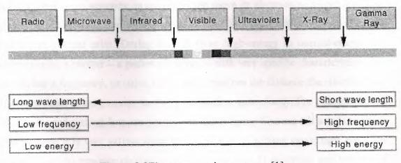
Figure 2.2 Electromagnetic spectrum. [1]
