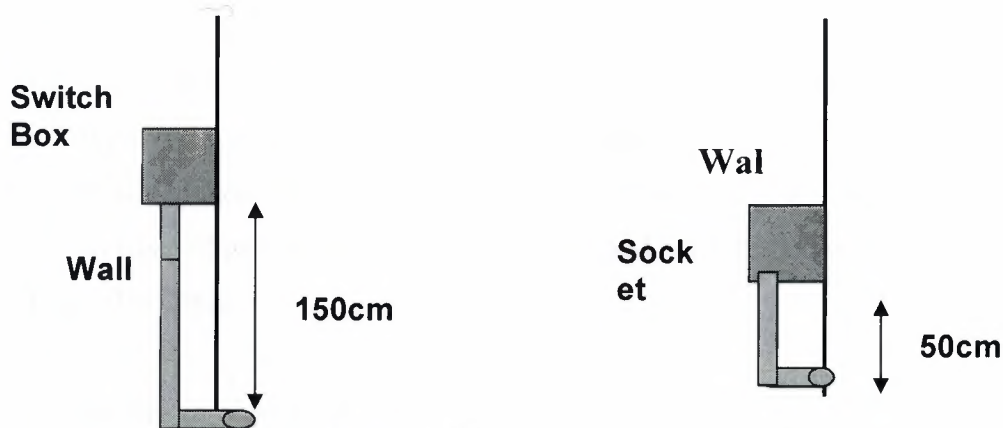
Figure 6. Height of switch and socket boxes
