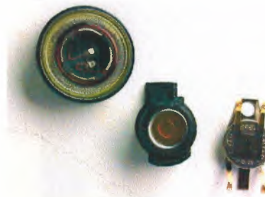
Figure 12.2 The cell phone speaker, microphone and battery backup.
