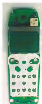
Figure 2.10 The display and keypad contacts.
