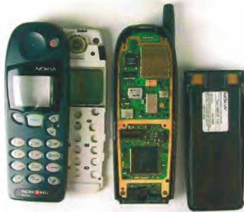
Figure 2.7 The various parts of a cell phone.
