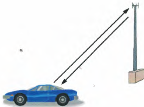
Figure 2.3 In duplex radio, the two transmitters use different frequencies, so both parties can talk at the same time. Cell phones are duplex
