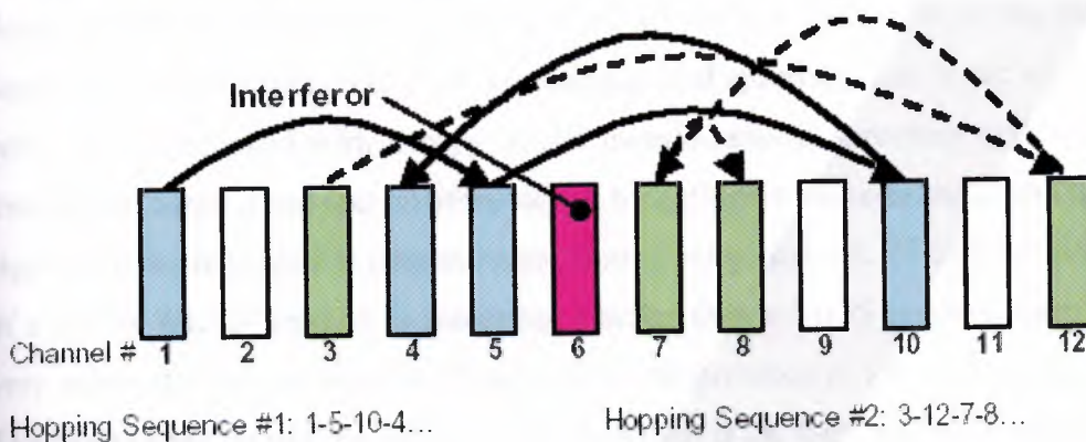
Figure 4.2: Frequency Hopping Spread Spectrum
