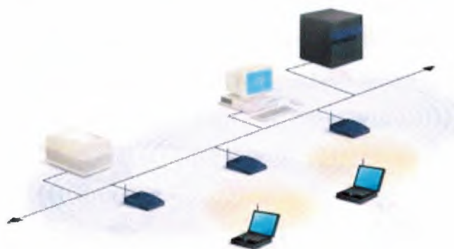
Figure 2.5 : Multiple access points and roaming
