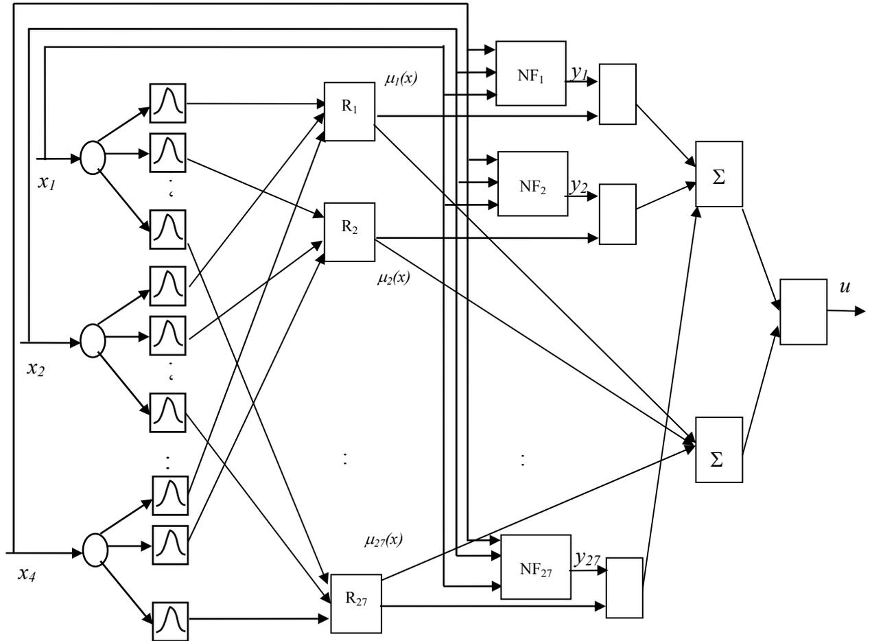
**Figure 4.2** The structure of NNFN based equaliser
