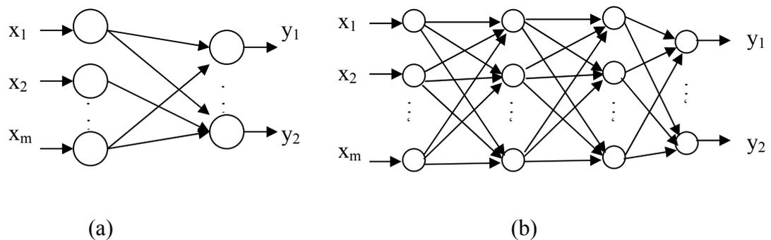
**Figure 3.5** (a) a single layered, (b) a simple multilayer neural network
