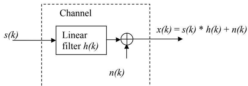
**Figure 2.4** The linear filter channel with additive noise [59]
