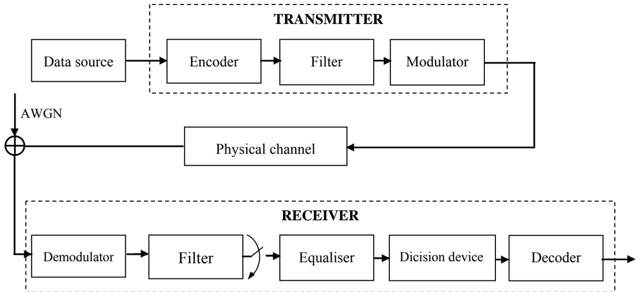
**Figure 2.2.** Architecture of a digital communication system. [31]
