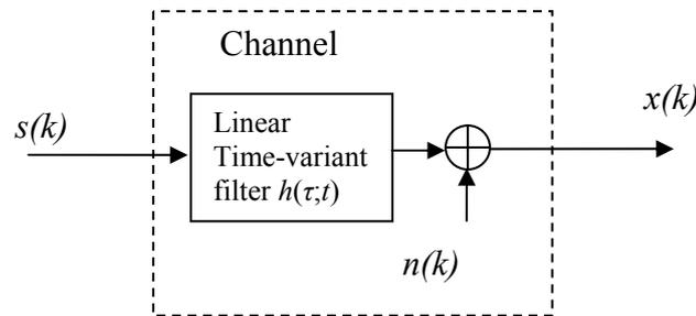
**Figure 2.5** Linear time-variant filter channel with additive noise [61]
