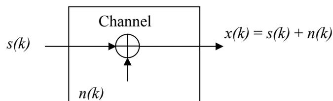
**Figure 2.3** The additive Gaussian noise channel [59]
