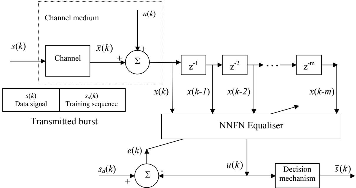
**Figure 4.1** The structure of the equalisation system
