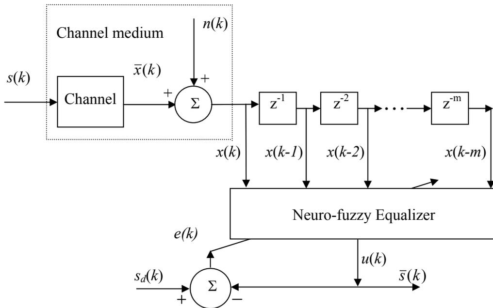
**Figure 2.6** Structure of a neuro-fuzzy equalisation system
