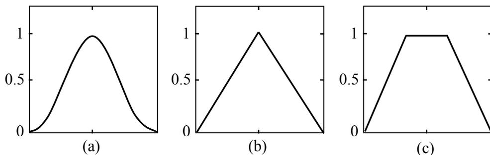
**Figure 3.2** Examples of membership functions (a) bell, (b) triangular, (c) trapezoidal
