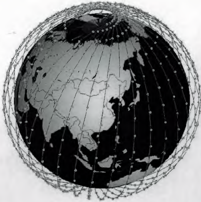
Figure 5.3 Teledesic Will Use a Large Number of LEO Satellites to Offer Access to Broadband Digital Transmission Telecommunications
