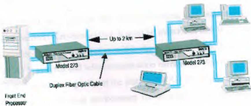
Figure 3-8: Model 273 realizing time division multiplexed data communications to a mainframe computer through its FEP.
