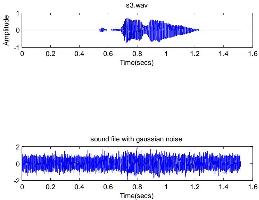
**Figure 7.17** Sound waveforms with and without large added noise (variance 0.04).
