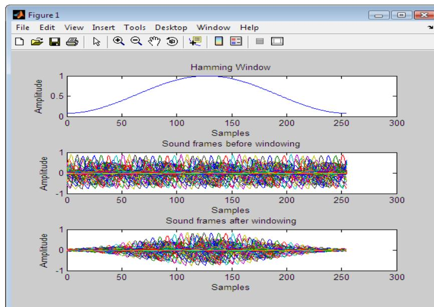
**Figure 7.10** Typical output from the program showing the effects of windowing
