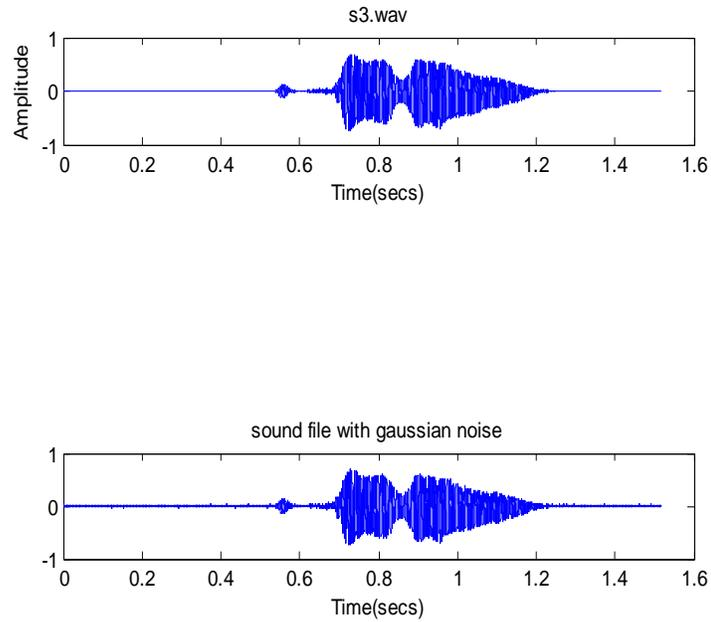
**Figure 7.16** Sound waveforms with and without larger added noise (variance 0.01)
