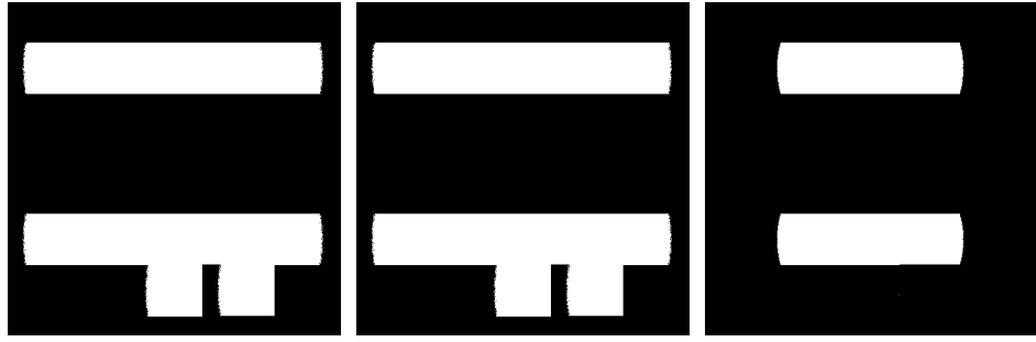
(a) binarization of 4.6(a) by Otsu Method (b) binarization of 4.6(b) by Otsu Method (c) binarization of 4.6(a) by Kittler and Illingworth Method
