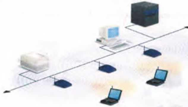
Figure 1.5: Multiple access points and roaming
