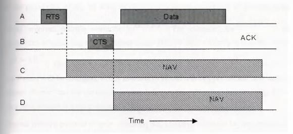
Figure 2.7: The use of Virtual Channel Sensing using CSMA/CA.
