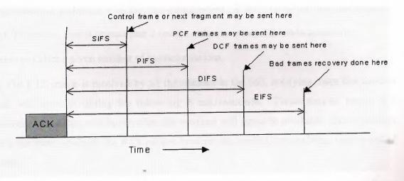
Figure 2.9: Interframe spacing for 802.11.
