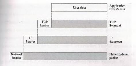
Figure 2.2: Protocol Data Units In The TCP/IP Architecture
