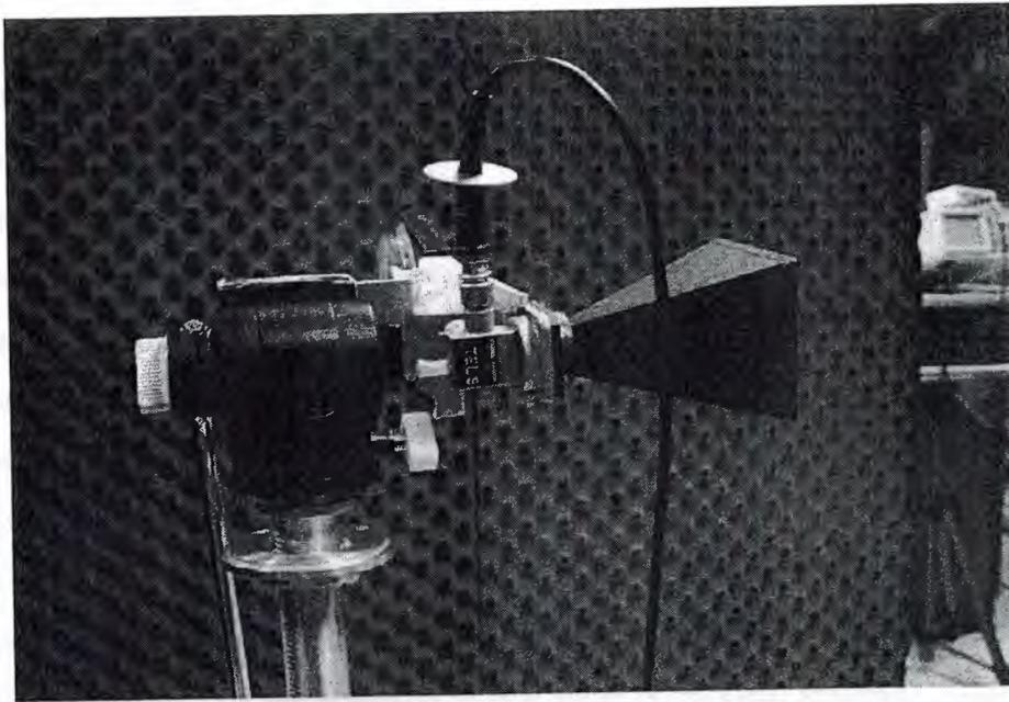
**Figure 1.9** 18-dBi X-band pyramidal horn antenna on swivel mount.
