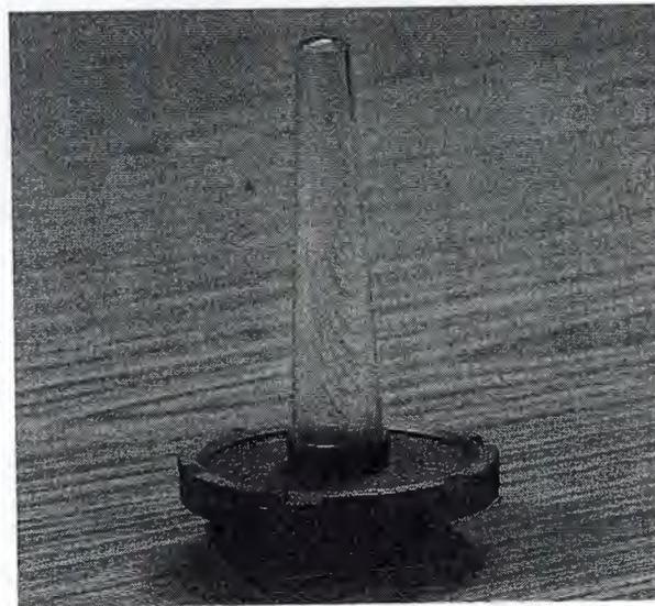
**Figure 1.6** Dielectric-rod ("polyrod") X-band antenna.
