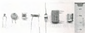
Figure 1.31 Capacitor materials. From left: multilayer ceramic, ceramic disc, multilayer polyester film, tubular ceramic, polystyrene, metalized polyester film, aluminum electrolytic. Major scale divisions are in centimetres.
