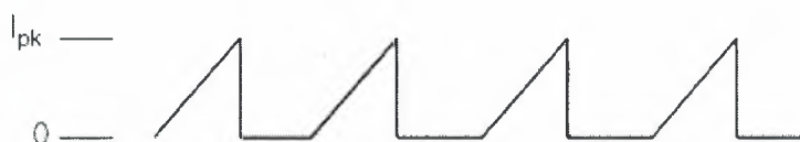
Fig. 10. Discontinuous Mode, Flyback Power Supply I_p (Primary Current)
