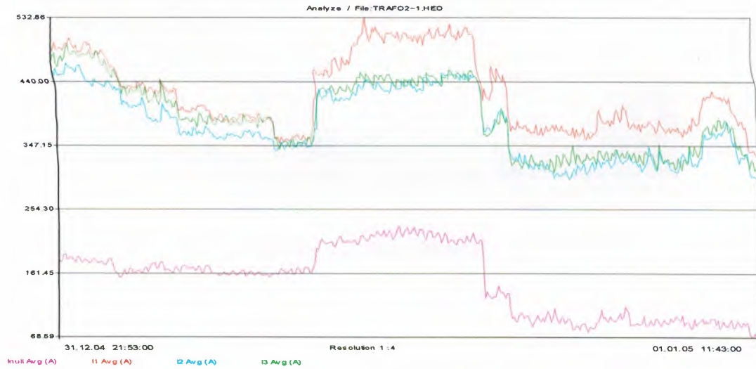
Fig 4.3.6 Transformer -2 Phaze currents & neutral current
