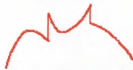
Figure 1.6.1 – Piecewise continuous waveform
