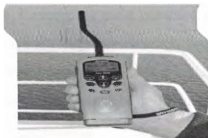
Figure 2.1: Handheld wireless radios such as this Maritime VHF radio transceiver use electromagnetic waves to implement a form of wireless communications technology.
