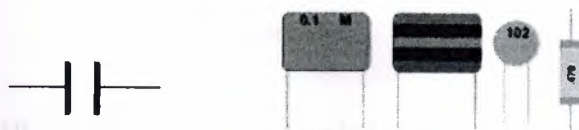
Figure 1.9 Circuit symbol & examples of the unpolarized capacitor.
