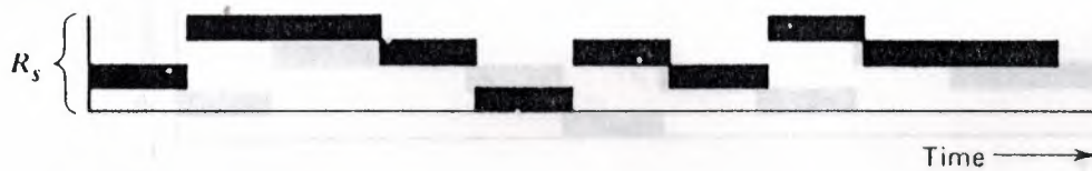
Fig.4.2 Illustrating Slow-Frequency Hopping
