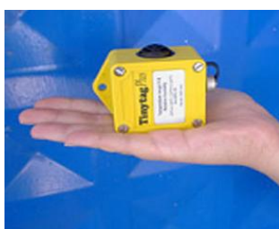
Fig. 3. A data-logger used during the environmental monitoring activities.
