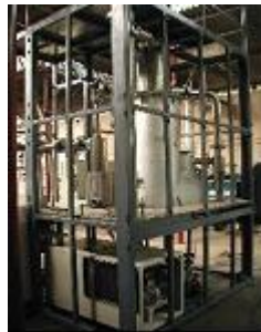
Figure 1. 20 kw Gasification system being tested at IPT/USP CENBIO, [3].
