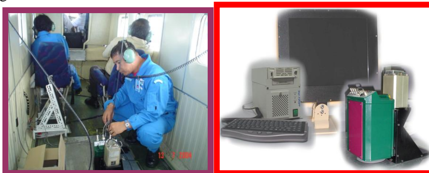
Fig. 2. Mounting the UPM-APSB sensor on-board the GAF N22B aircraft Fig. 3. The complete airborne system with a total weight of only 15 kg
