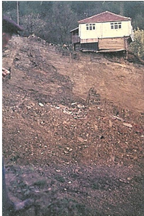
Figure 8 A portion of land which is displaced vertically about 5-6 meters due to landslide.
