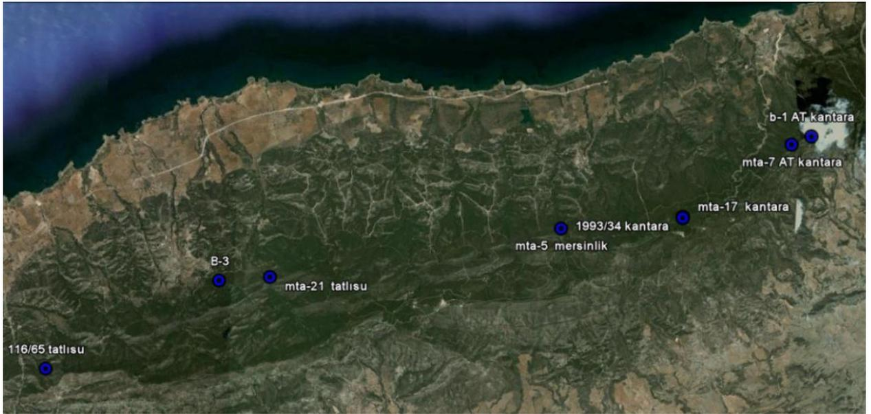
**Figure 3.77** Areal picture showing the locations of boreholes (from top view) in Tatlısu Kantara Region (scale, 1:125,000).
