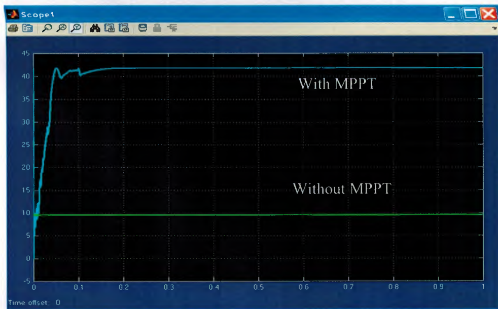
Case 1: R=50(\Omega) , I_r=1000 ( \text{W}/\text{m}^2 ), T= 25 (C).
