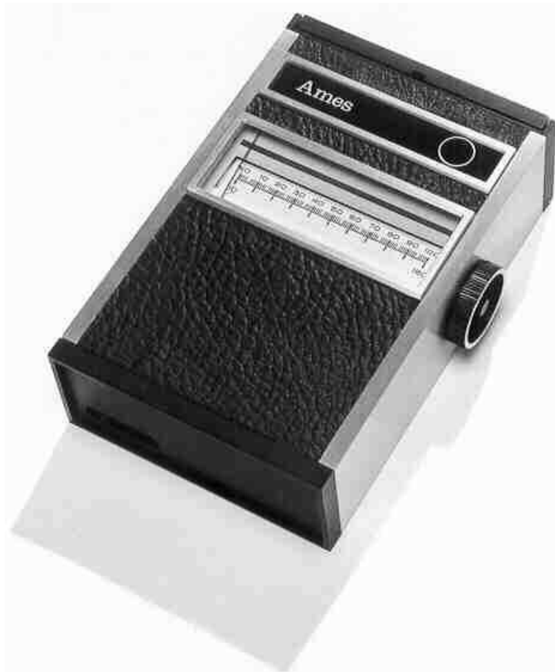
Figure 22: Ames Reflectance Meter, first glucose meter developed [11]
