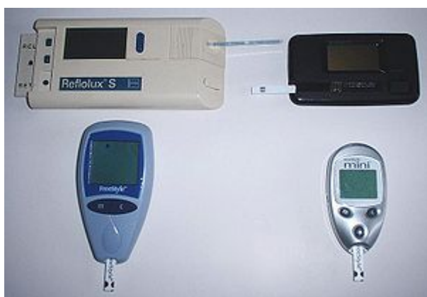
Figure 12: Four generations of blood glucose meter, c. 1993-2005. Sample sizes vary from 30 to 0.3 \mu l. Test times vary from 5 seconds to 2 minutes (modern meters typically provide results in 5 seconds). [14]
