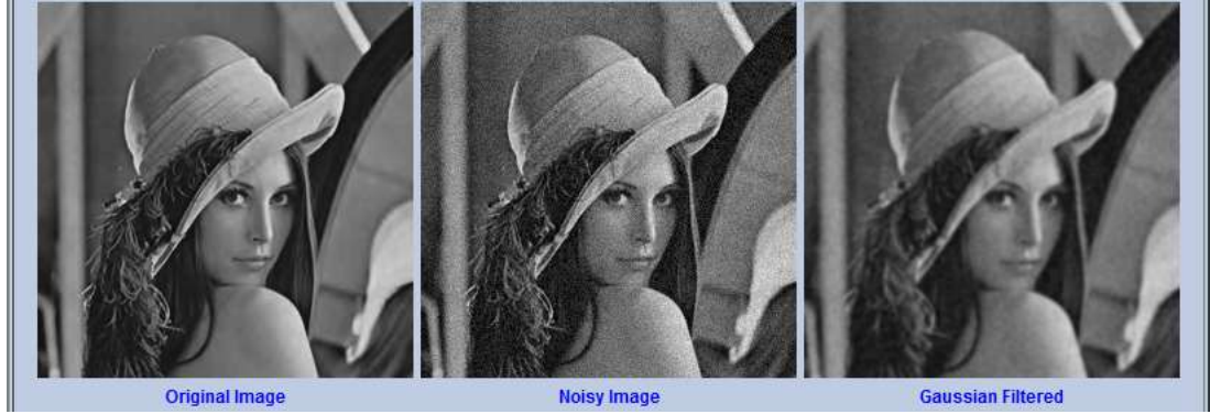
Figure 3.7 An example of Gaussian Smoothing Filter (Nixon, M., & Aguado, A., 2002).
