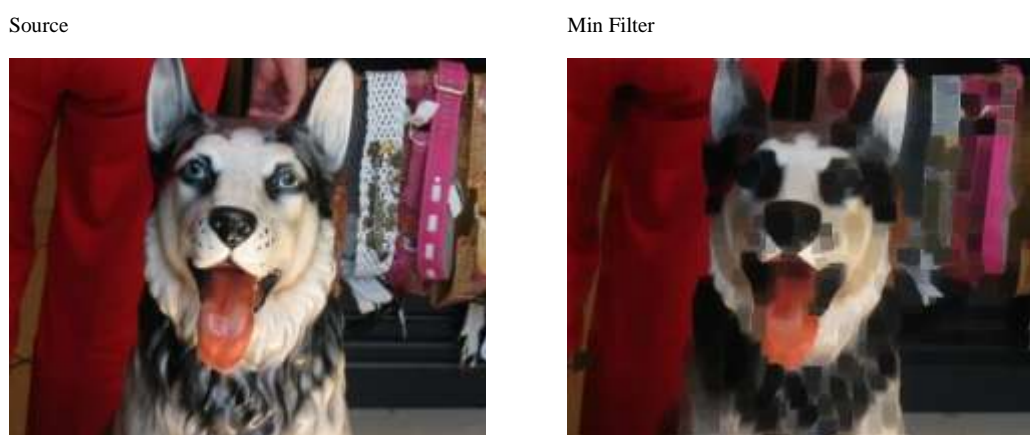
Figure 3.3. An example of Min Filter Operation (RoboRealm, 2005).
