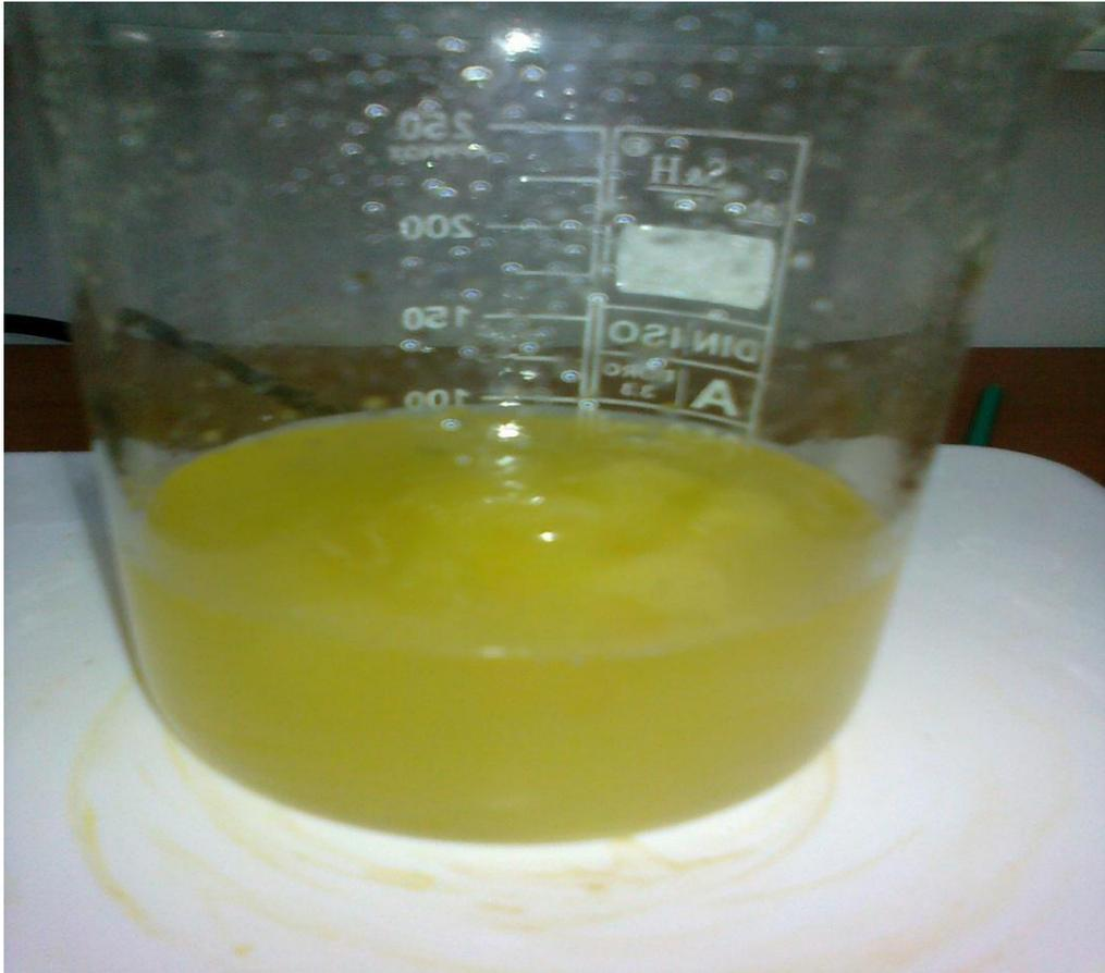
Figure 2.5: Silk fibers dissolving in the electrolyte solution
