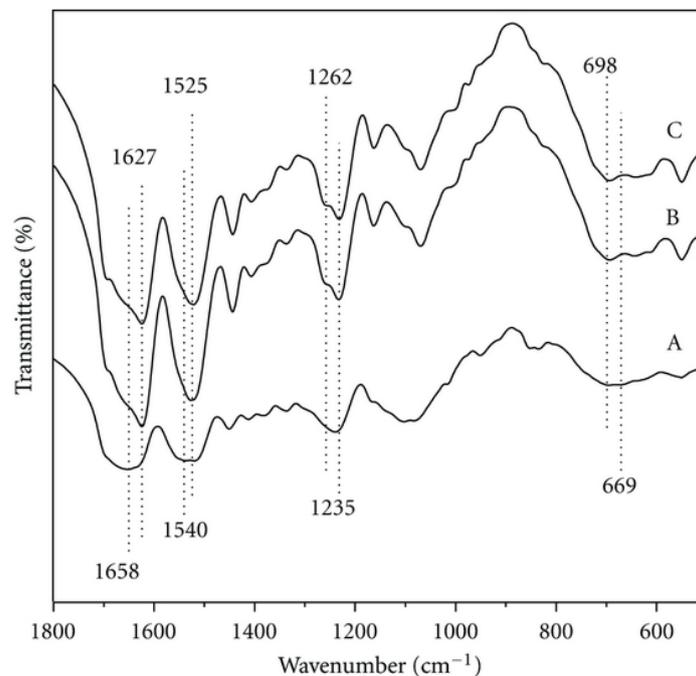
Figure 1.6: FTIR spectra of porous SF scaffold incubated with collagenase (Hu, (2012)).
