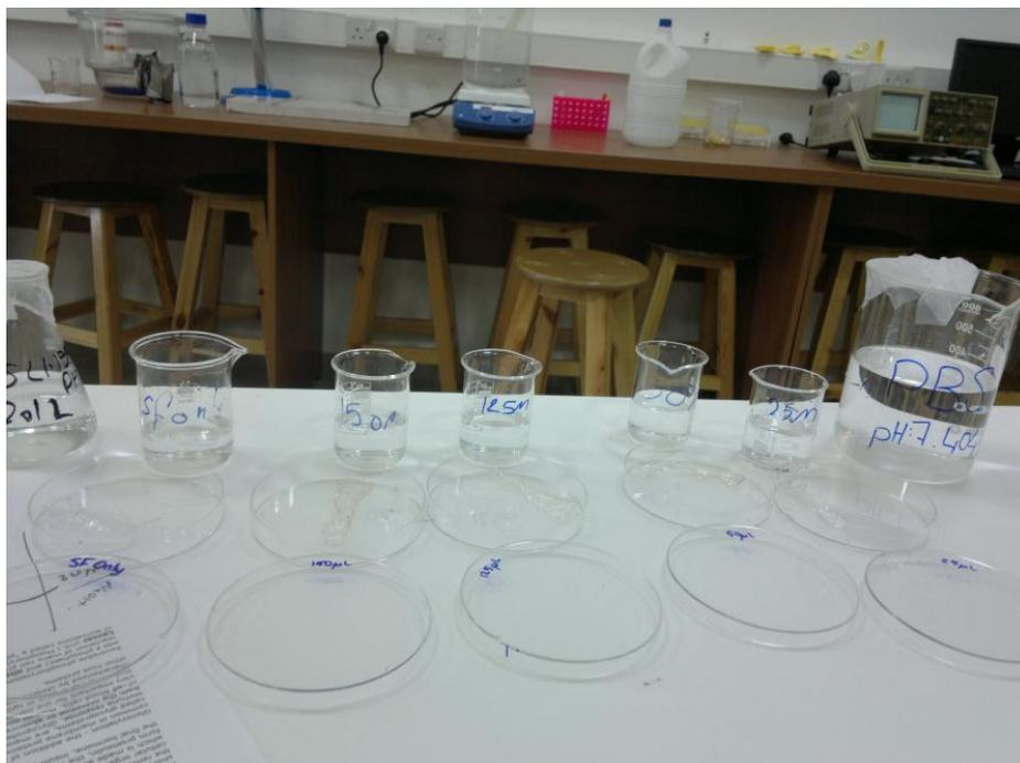
Figure 2.10: Swelling tests for the silk fibroin biofilms.
