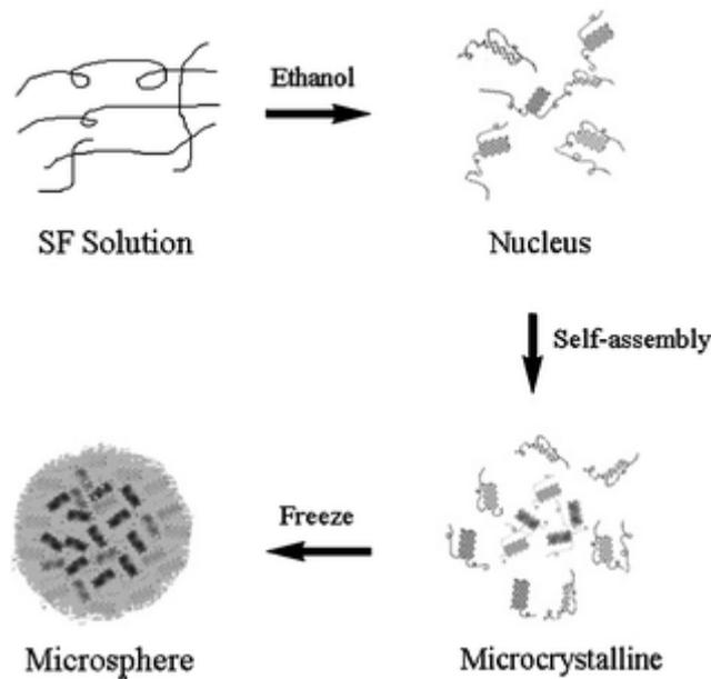
Figure 1.7: The preparation of regenerated SF microspheres (Cao et al, 2007).
