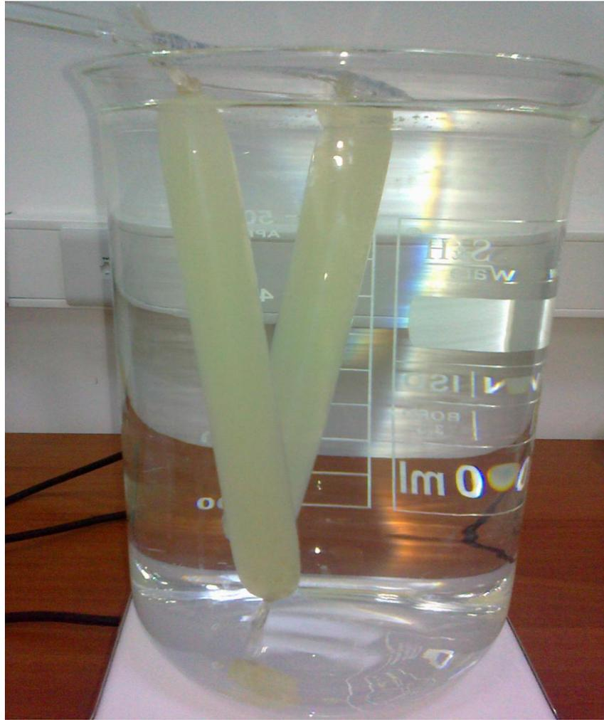
Figure 2.6: Dialysis of the aqueous silk fibroin with distilled water.
