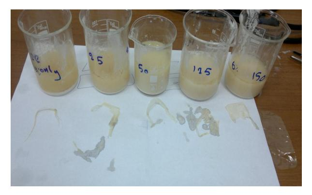
Figure 3.15: Biodegradation test for SF biofilms with protease enzyme.
