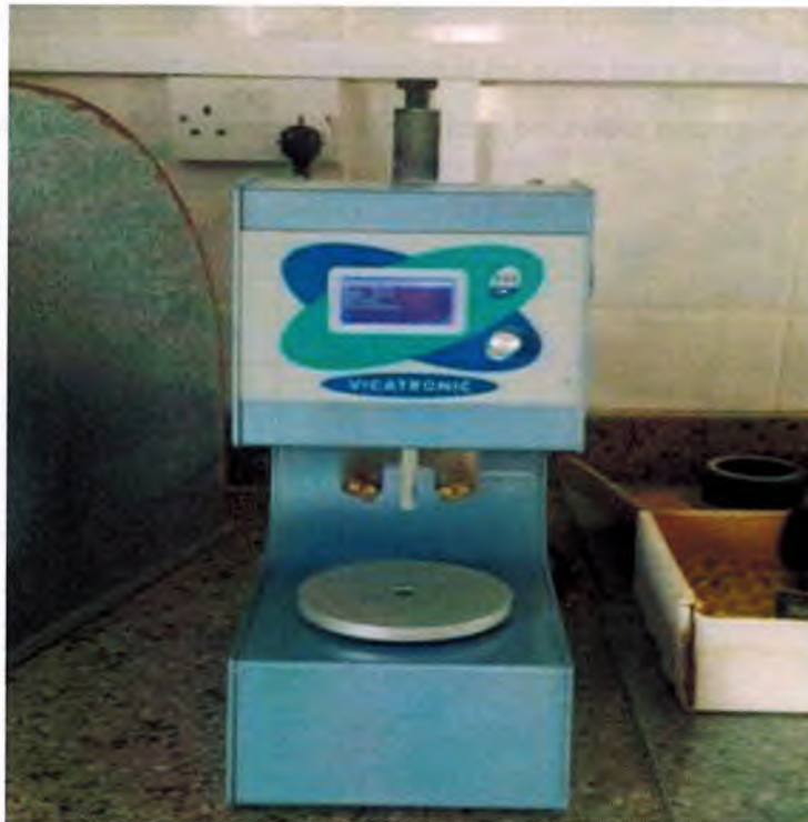
Fig 3.4: Vicat Apparatus used in this study
