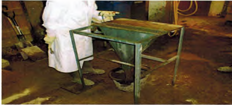
Fig 2.6: V-funnel test (Liu, 2009)
