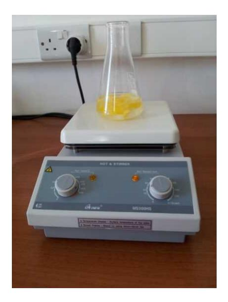
**Figure 2.2:** *Bombyx mori* cocoons in the degumming process in 0.1M Sodium Carbonate (Na<sub>2</sub>CO<sub>3</sub>) solution at the speed of 1.5 rpm at 75 °C
