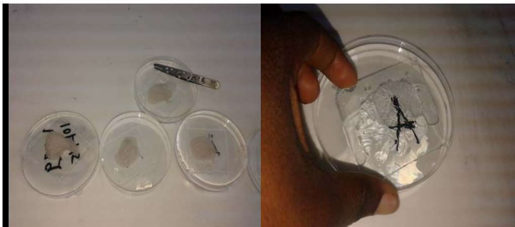
Fig 2.4(a) Cs-Urchin composite in distilled H 2 O 2.4(b) Pure chitosan swelling in distilled H 2 O
