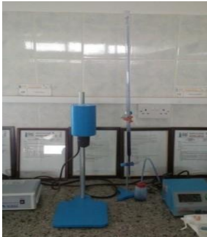
Fig 3.3: Methylene Blue test Apparatus Used in this study
