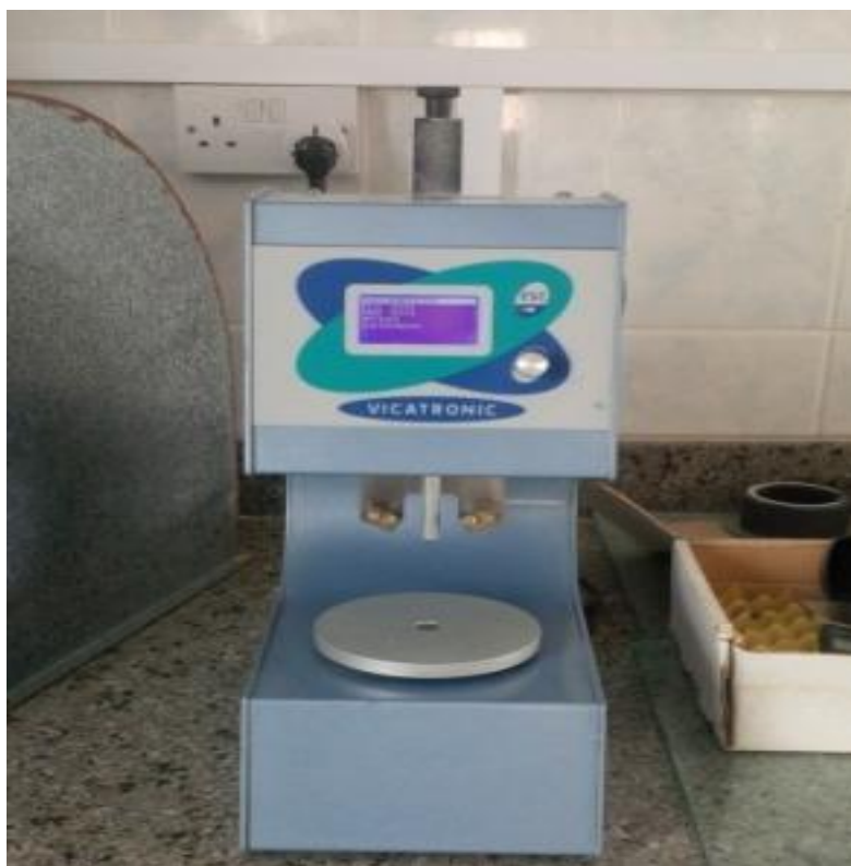
Fig 3.4: Vicat Apparatus used in this study
