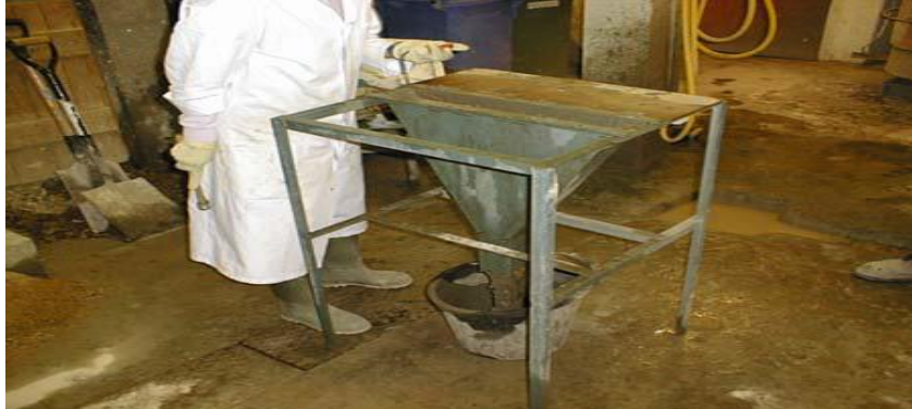
Fig 2.6: V-funnel test (Liu, 2009)
