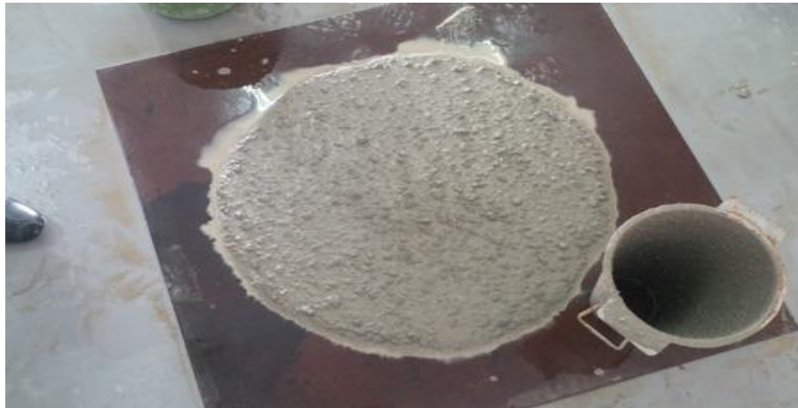
Fig 2.5: Slump flow test
