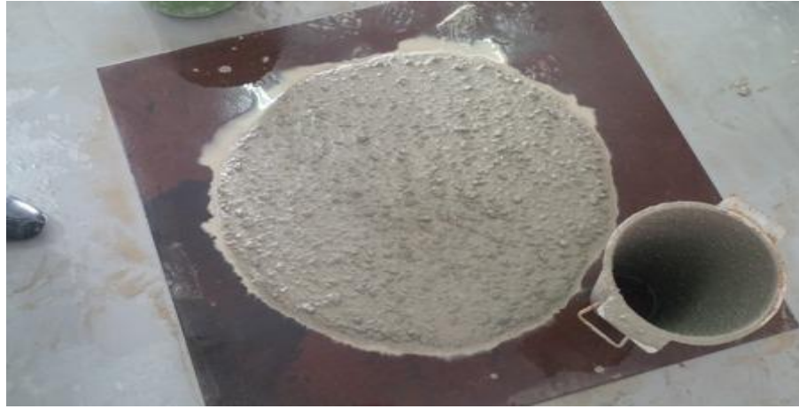
Fig 3.5: Slump flow test carried out in this study
