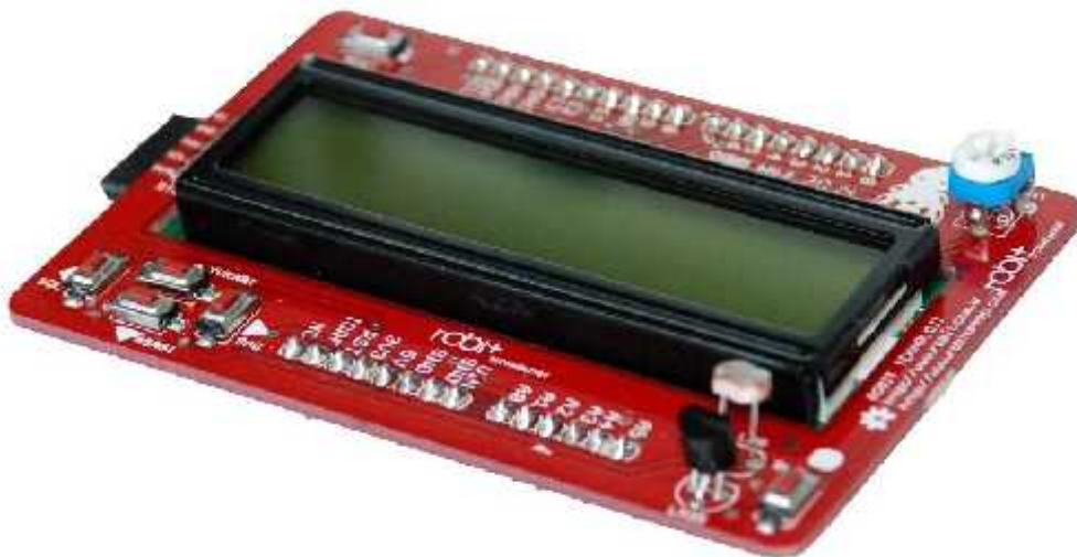
Picture 5.5: 2x16 LCD screen shield V2 for 'Arduino Uno R3'
