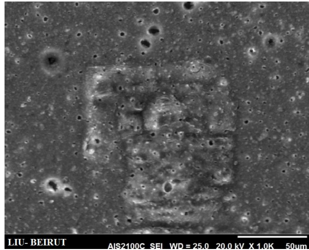
Figure 5.6: SEM image of porous PMMA at 50μm
