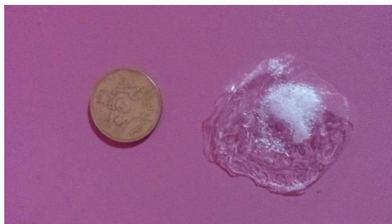
Figure 4.20: PDMS cured at room temperature for ( V_{\text{PDMS}} : V_{\text{Gluteraldehyde}} ) : (1:11) ratio application
