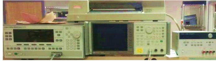
Figure 3.8: Network analyzer (Agilent HP 80350A 8756A-10 MHz to 40 GHz).
