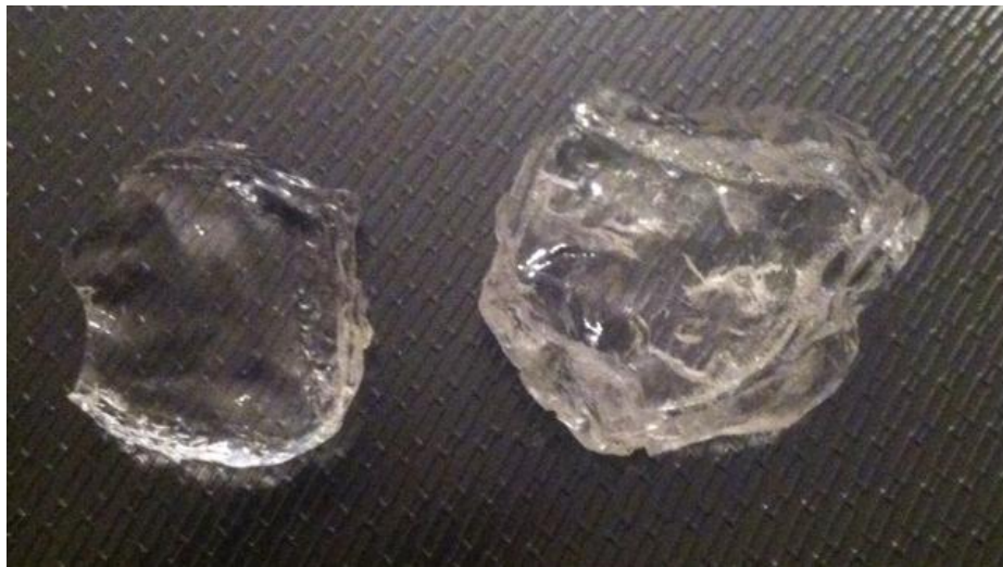
Figure 5.8: On the left the mold PMMA, on the right the completing porous cured PDMS similar to silicon
