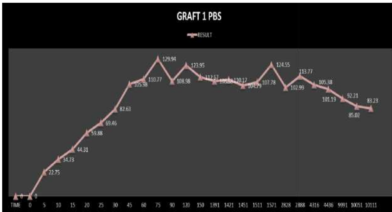
Figure-12:Swelling Test for Phosphate Buffer Saline of Graft 1
