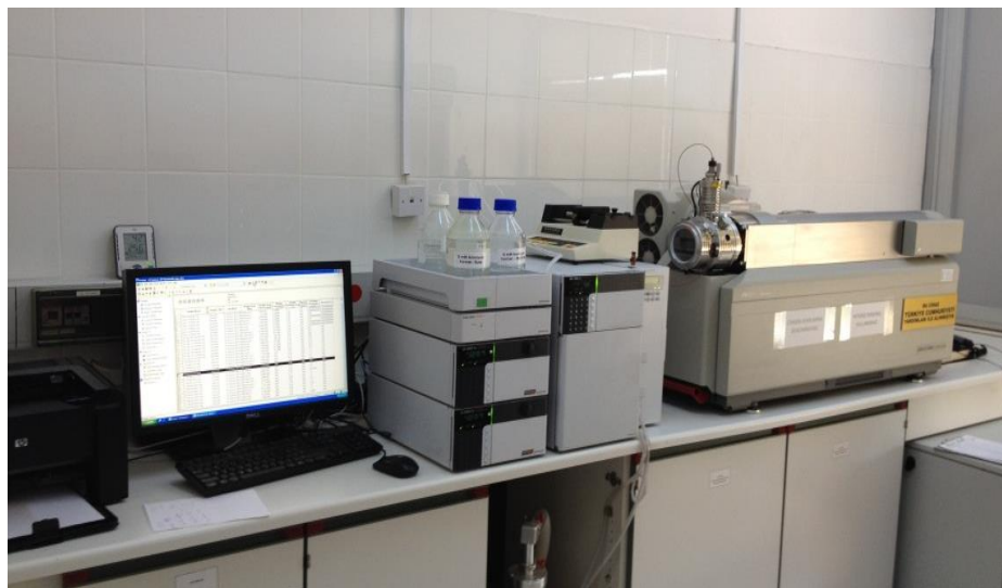
Figure 2.2: Liquid chromatography with mass spectrometer
