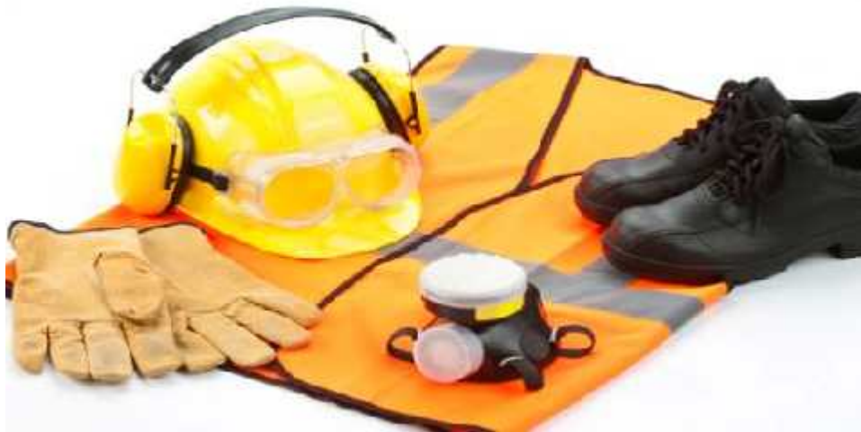
Figure 4.5: Typical Personal Protective Equipment (Oregon OSHA, 2011)
