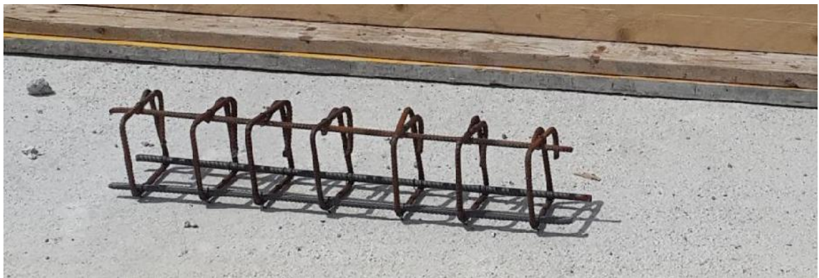
Figure 4.6: Internal Reinforcement of Group 2 Beams
