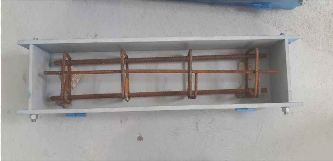
Figure 4.4: Internal Reinforcement of Group 1 Beams
