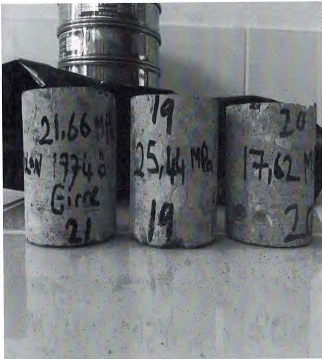
Figure 3.2: Sample of Drilled Cores from Existing Buildings
