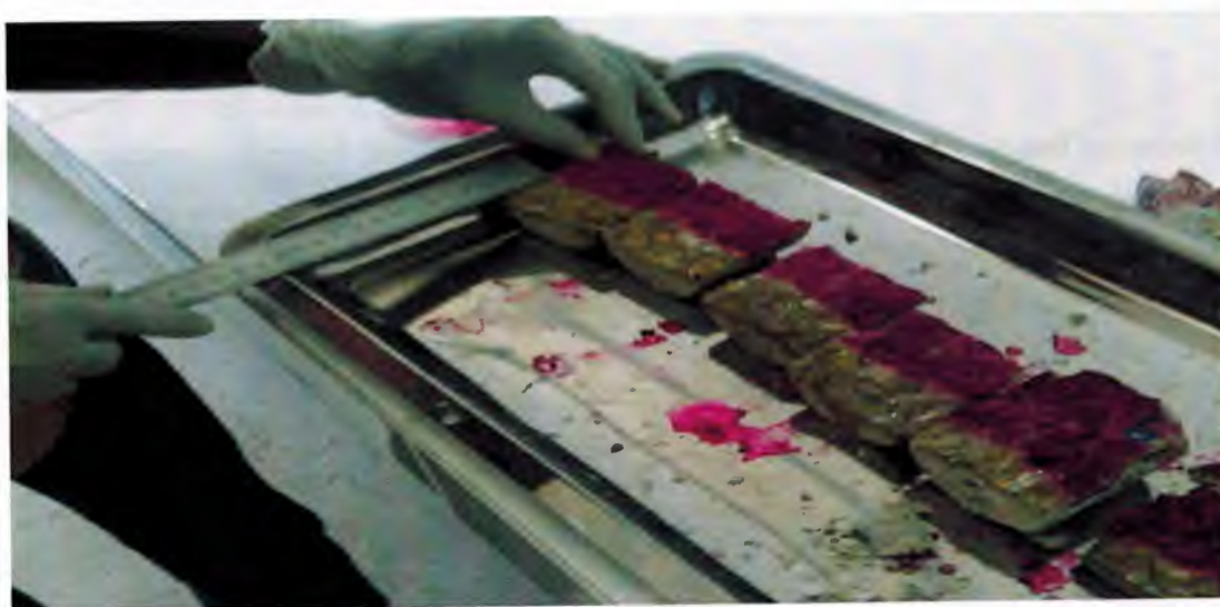
Figure 3.4: Measuring Carbonation Depth with Steel Ruler
