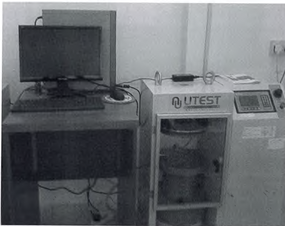
Figure 4.10: The Wood Test Compressive Machine [NEU Civil Lab]
