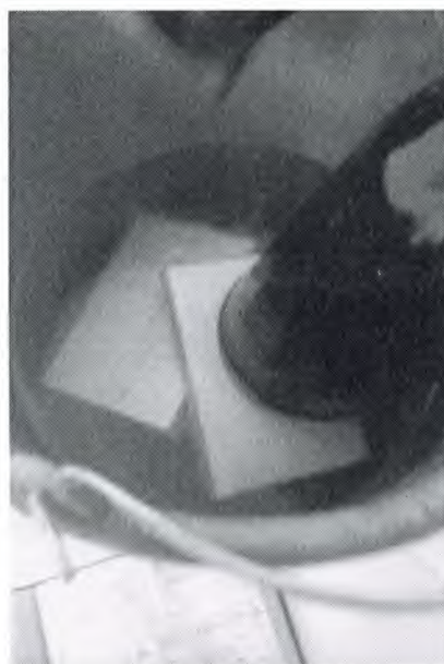
Figure 4.9 The wood soaked for 2.4 hours
